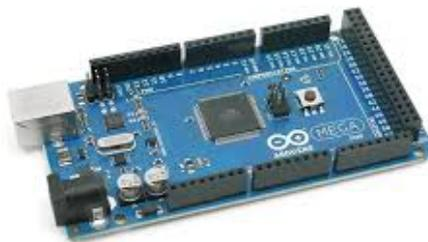
Figure 5.5: Arduino Mega 2560
