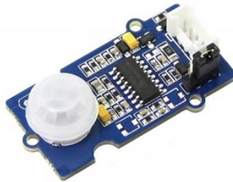
Figure 5.12: PIR motion sensor
