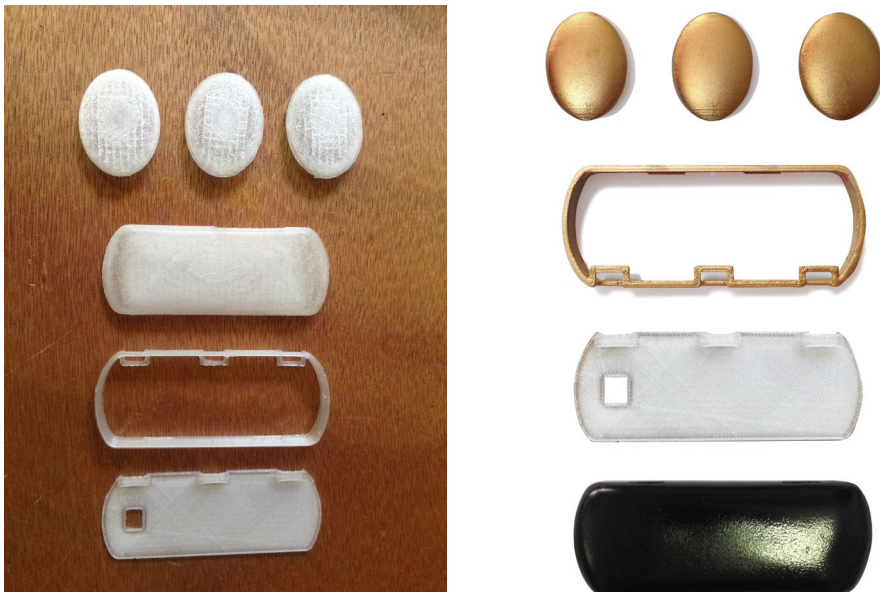
Fig. 7.15: The parts made by 3d printing. Left: before surface treatment; Right: After surface treatment.
