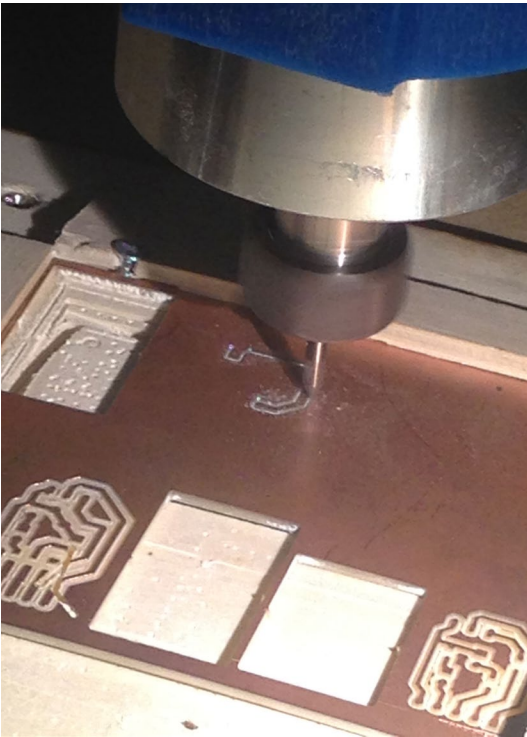
Fig. 7.12: The rapid PCB cut by CNC machine.
