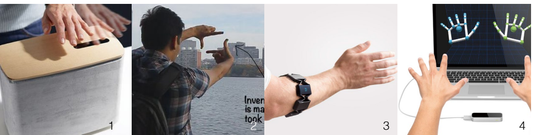
Fig. 5.9: Non-contact gestures examples. 1. P.A.C.O. by Digital Habits; 2. SixthSense; 3. Myo gesture control armband; 4. Leap motion controller.
