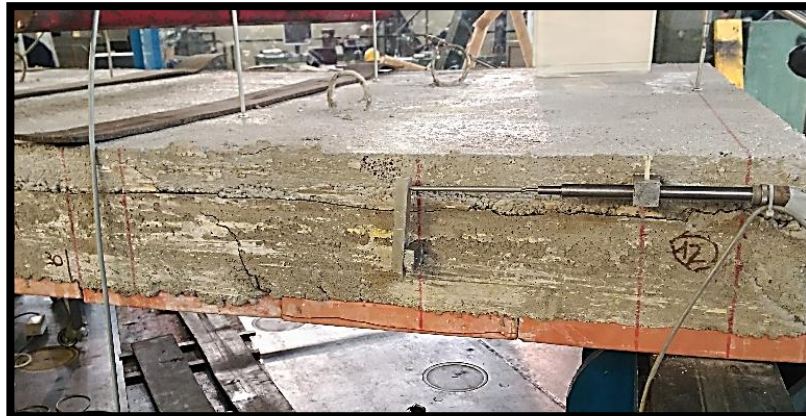
Figure 35. Failure of the second consolidated floor slab of h = 16 + 5 cm. (Source: Laboratory image)
