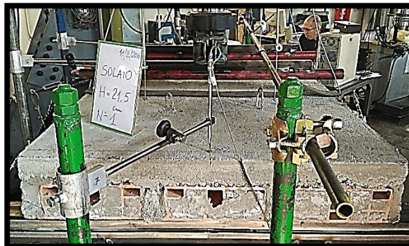
Figure 22. Instruments to measure the deflection. (Source: Laboratory image)
