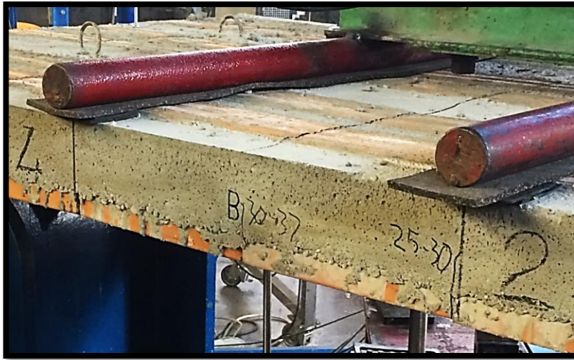
Figure 28. Failure of the first non – consolidated floor slab of h = 12 cm. (Source: Laboratory image)
