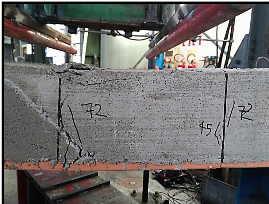
Figure 89. Lateral failure of the second specimen of h = 16 cm. (Source: Laboratory image)
