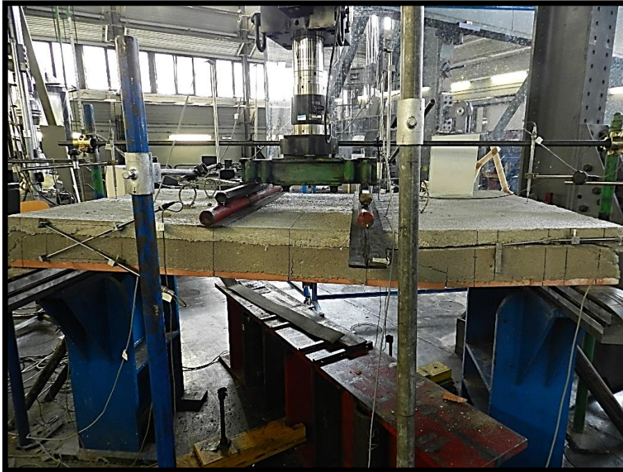
Figure 94. Failure of the first specimen of h = 21 cm. (Source: Laboratory image)
