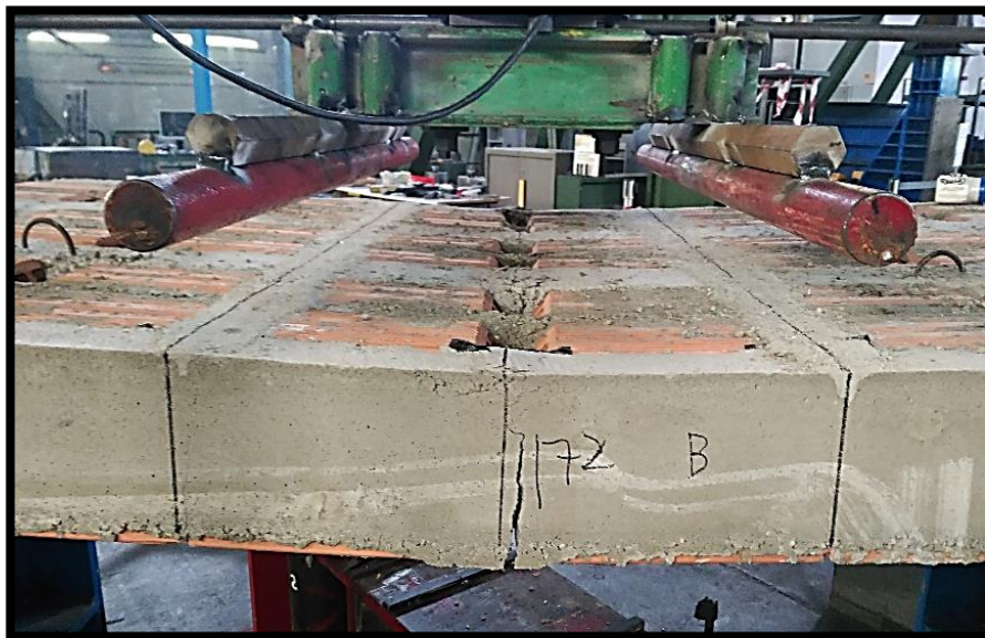
Figure 31. Failure of the second non – consolidated floor slab of h = 16 cm. (Source: Laboratory image)
