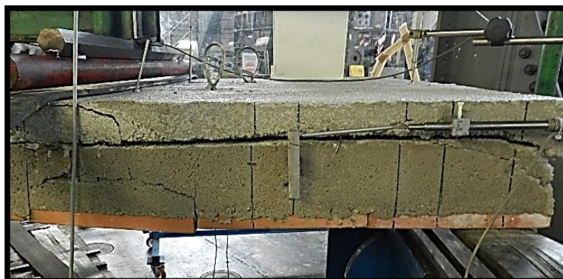
Figure 34. Failure of the first consolidated floor slab of h = 12 + 5 cm. (Source: Laboratory image)
