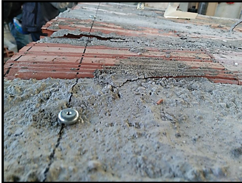
Figure 86. Top failure of the second specimen of h = 12 cm. (Source: Laboratory image)
