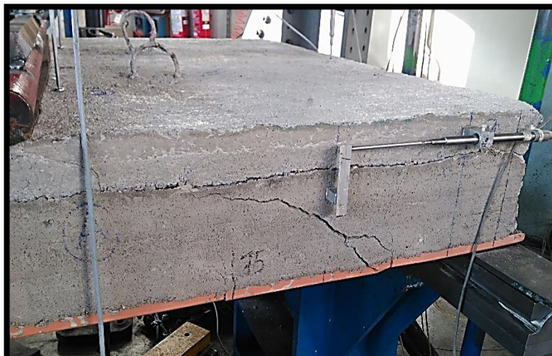
Figure 32. Failure of the first consolidated floor slab of h = 12 + 5 cm. (Source: Laboratory image)
