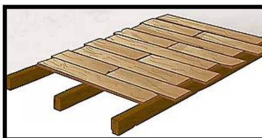
Figure 2. One – way floor slabs with one frame with wooden plank. (Source: Leca)
