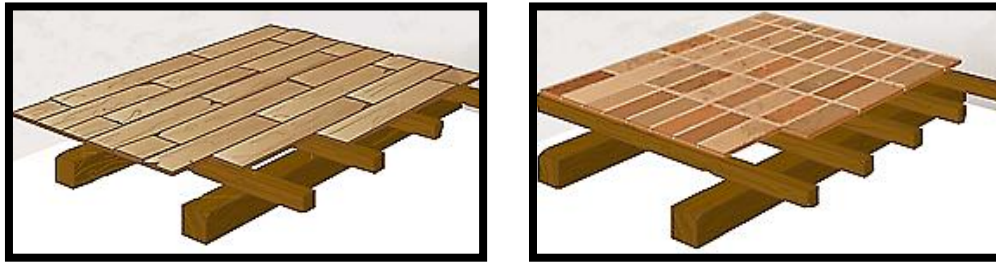
Figure 3. Two – way floor slabs with both wooden and brick plank. (Source: Leca)
