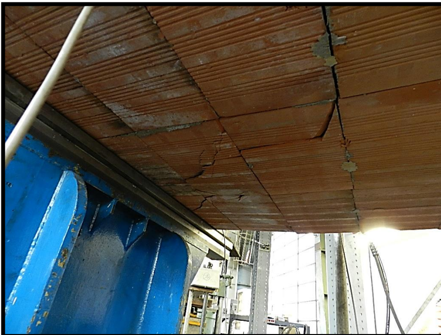
Figure 95. Bottom failure of the first specimen of h = 12 cm. (Source: Laboratory image)
