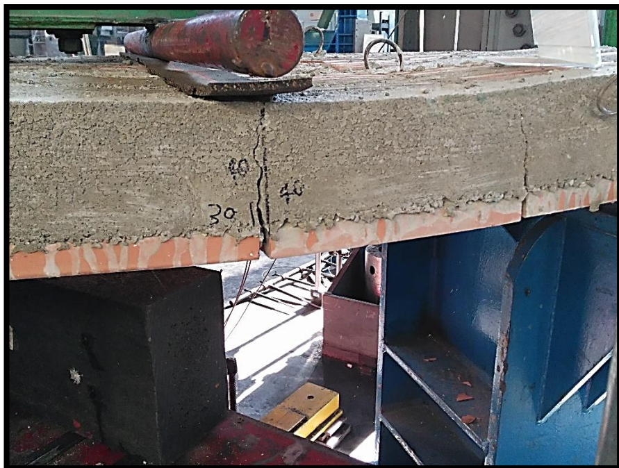
Figure 85. Lateral failure of the second specimen of h = 12 cm. (Source: Laboratory image)
