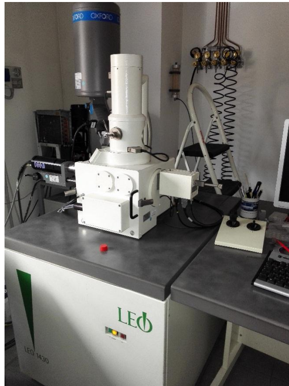
Fig.3.15. SEM model LEO 1430 used to perform SEM analysis.
