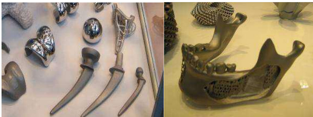
Fig.1.9: Example of prosthesis production via selective laser fusion (on the left) and maxillofacial implantology (on the right).
