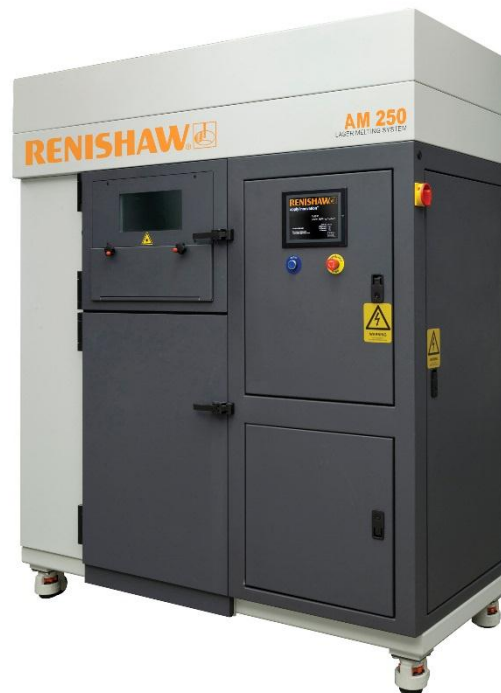
Fig.3.2: Renishaw AM250 used to fabricate the samples.
