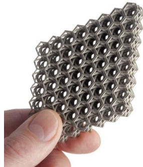
Fig.1.1: Example of reticular structure realized via laser melting technique. This type of structure guarantees the lightness satisfying the mechanical properties of the component ( www.renishaw.com ).
