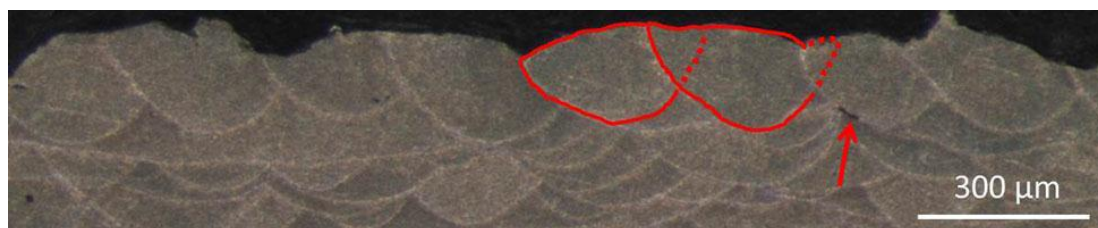
Fig.1.20: Close up of track segments, showing the dimensions of the half-cylindrical melt pools. Early formation of a defect can be seen marked by the arrow (I. Rosenthal, 2014).
