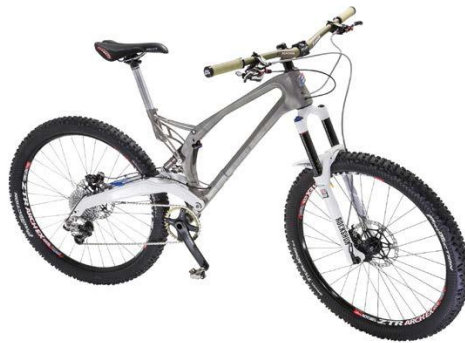
Fig.3: Mountain bike was developed by Renishaw and Empire Cycles using additive manufacturing, and topologic optimization ( www.renishaw.com ).
