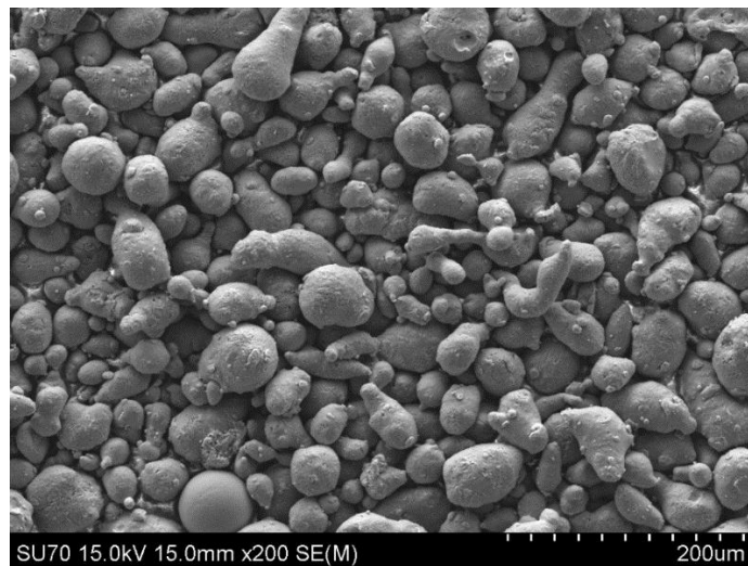
Fig.4.1: SEM image of the gas-atomized powder.
