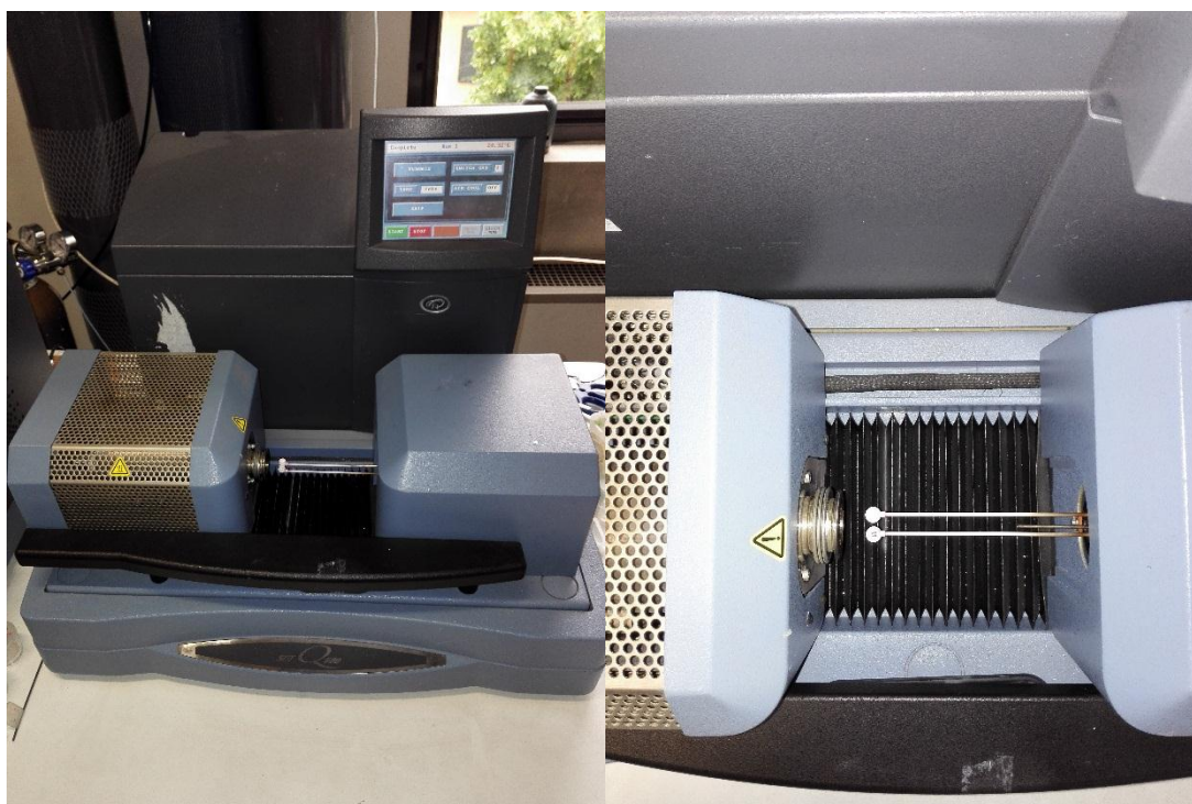
Fig.3.18: On the left, the Q600 used for the DTA analysis, on the right the two pans (one empty and one in which the analyzed sample is placed).
