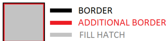
Fig.3.6: Definition of the three different scanning zones ( Borders , Additional Border and Fill Hatch ) of a square section on x-y plane.
