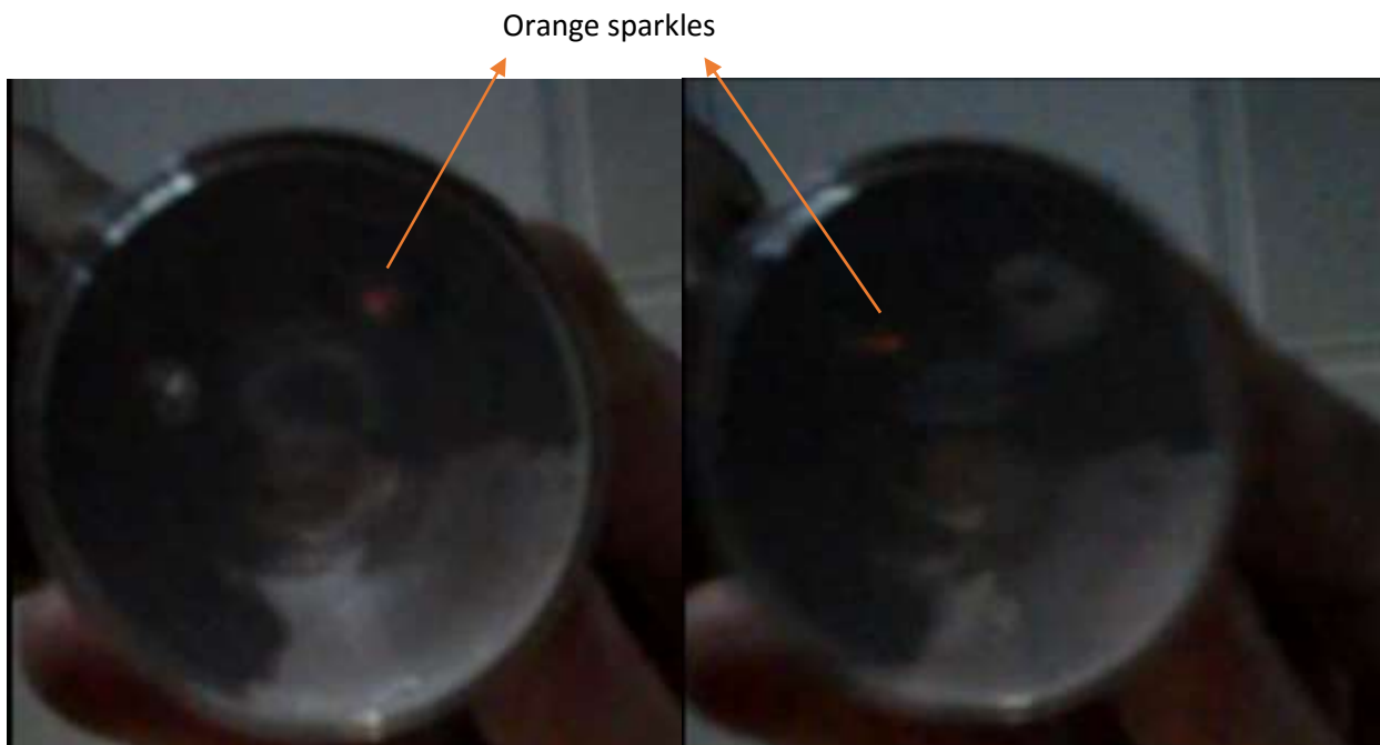
Figure 4.14. Orange light emission from the EML ZnS/Al powders produced by solid state reaction on the left hand side and solution processes.
