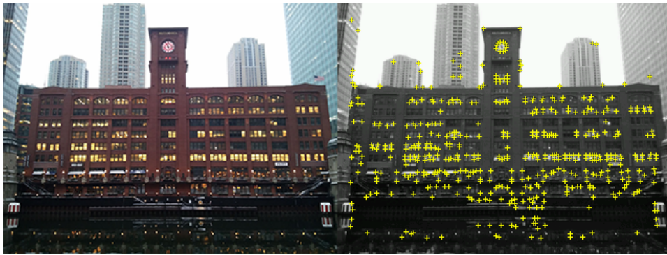
Figure 3.3: Sample image uploaded to Vuforia Target Manager: on the left we can see the original picture, on the right the image is turned to grayscale and features are rendered on top of it.
