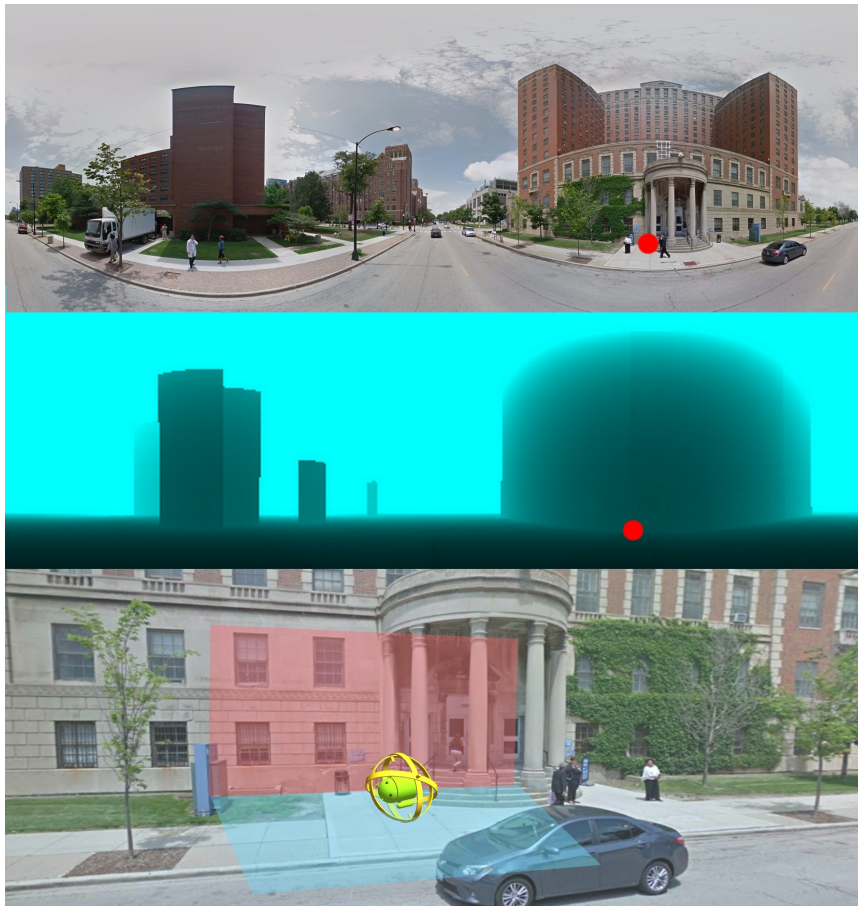
Figure 4.13: Implementing a web-based editor by leveraging Google Street View imagery. In the figure above it is possible to observe a sample panoramic image (top) and its relative computed depth map (middle). The depth information is used to allow a more precise positioning of the virtual objects in the real world (bottom), which can simply be dragged into the scene and then moved, scaled or rotated.
