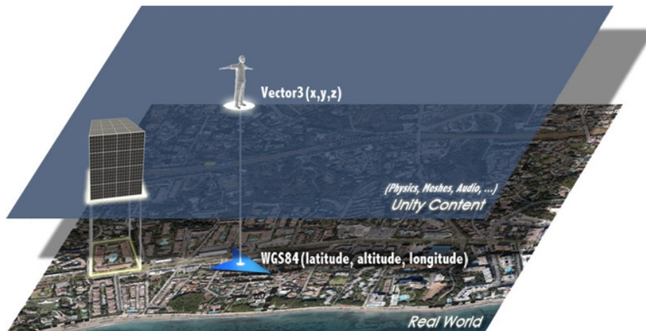
Figure 3.1: Mapping the two worlds. While a user walks in the real world, a virtual camera moves and rotates accordingly in the virtual scene, defining which elements need to be rendered on top of the live camera stream of the player’s device [53].
