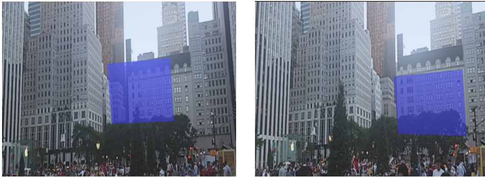
Figure 5.12: In the above sample scenario, SensorCamera (dual camera approach, left) and SLAMCamera (triple camera approach, right) extended tracking methods are compared in a sample situation in which the user has lost a tracked fiducial (a statue - not visible in the figure) and then rotated his mobile phone clockwise along the vertical axis by about 80^\circ . In the left image, we can notice how larger rotations in an urban environment can be affected by sensor unreliability. Despite in Chicago 0,0 the addition of the SLAMCamera appears to slightly increase the robustness of the tracking, eliminating the magnetic interferences that could limit the accuracy of the SensorCamera, it cannot however replace the ARCamera: in order to obtain a reasonable image overlay, we still need to leverage the presence of a geolocated fiducial.
