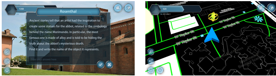
Figure 5.10: On the left, an example of a simple puzzle appearing on screen after a team reaches a virtual object. On the right, a sample map view showing the user approaching his next challenge, represented by an animation on the map (which may differ from the virtual object that will be shown in the camera view); the light blue element on the upper-right corner is instead a virtual sound zone – a particular type of virtual object that emits a sound whose intensity is proportional to the its distance from the player.
