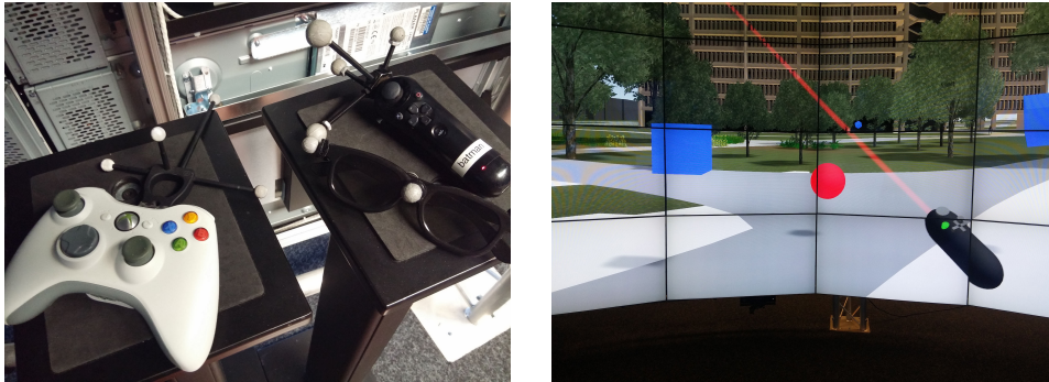
Figure 4.4: In the image on the left, it is possible to observe the 3D glasses that need to be worn by the user of the editor application and the two available controllers. On the right, the model of the Wand controller is shown on screen: by pressing the 'X' button, the user can generate a ray to facilitate the selection of objects.
