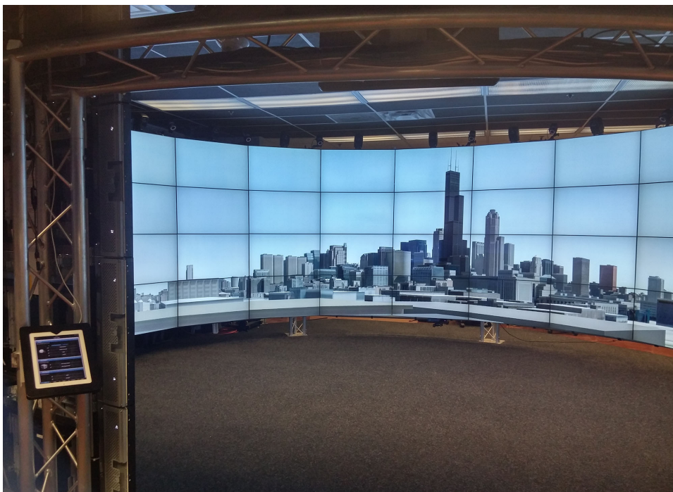
Figure 4.2: The 3D model of the city of Chicago that we will use for our experiments. The scale of the model is approximately 1 to 1, so that one unit in virtual space corresponds to one meter in the real world.
