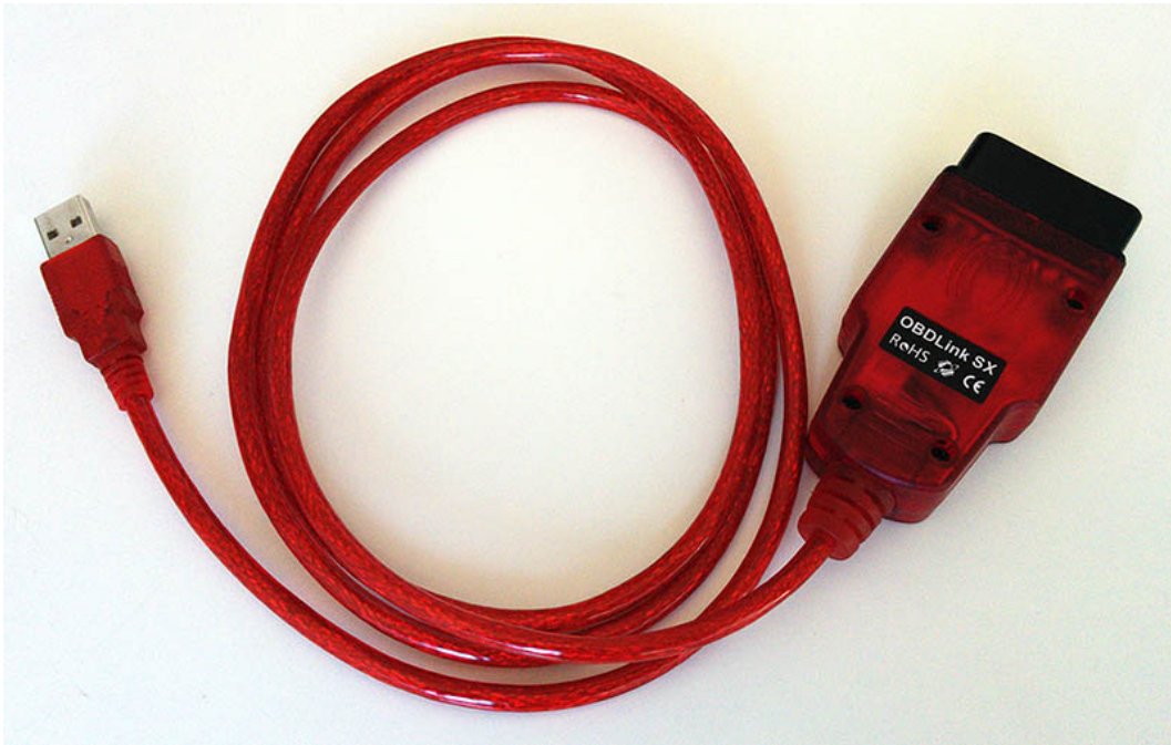
Figure 5.5: The Scantool OBDLink SX USB-to-OBDII cable.
