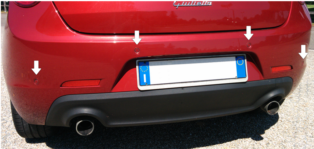
Figure 5.3: The parking sensors of the Giulietta, located on the rear bumper.
