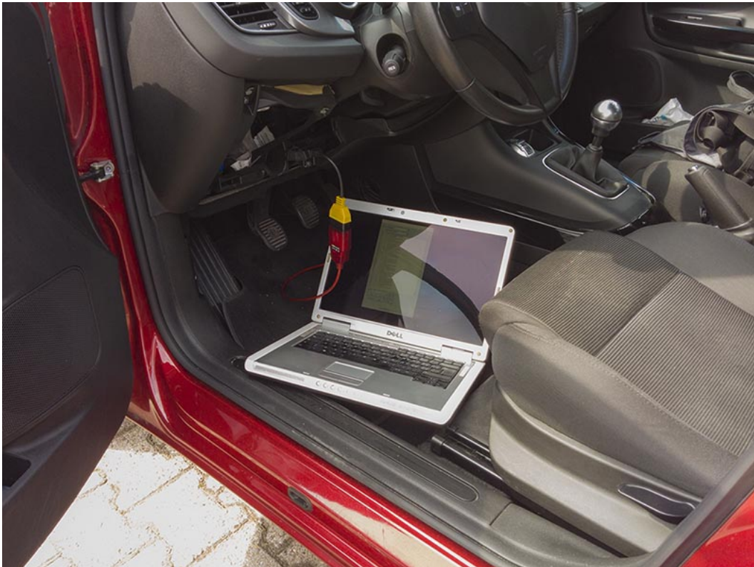
Figure 5.7: The capturing of the Giulietta CAN traffic via the OBDLink SX.
