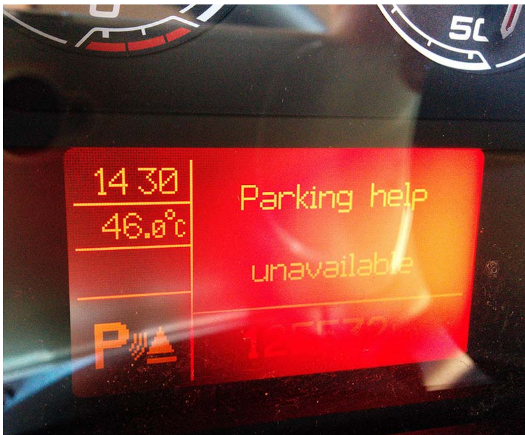
Figure 5.17: The parking sensors malfunction reported on the instrument panel cluster display.
