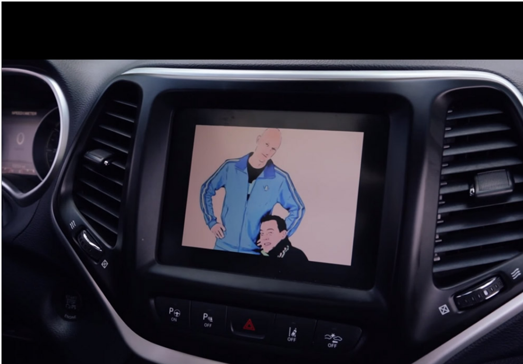
Figure 6.1: The remotely compromised Harman Kardon Uconnect system of a 2014 Jeep Cherokee [83].
