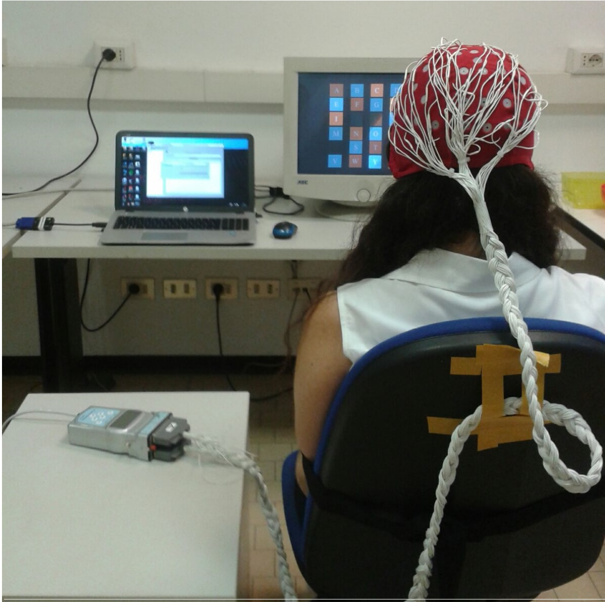
Figure 3.6: A view of the experimental setup. Presentation projects the scenario on a CRT screen and the subject is strapped to the chair in front of the monitor.
