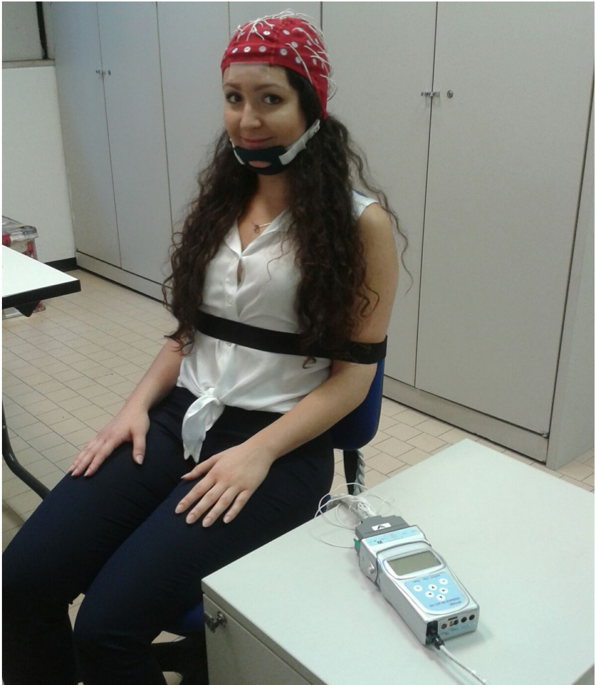
Figure 3.5: A view of the experimental setup. In particular, a clear image of the cap and the straps, plus the wired headbox.
