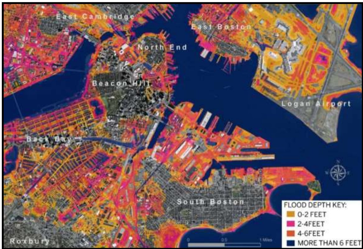
Figure 3-10: Boston Flooding with 2.5 Feet Sea Rise & 5 Foot Storm Surge (Globe Graphic – UMass Boston, Dr. Ellen M. Douglas)
