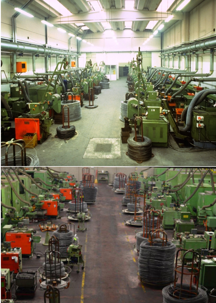
Figure 4.1: The heading machines floor of 2 screws production environments
