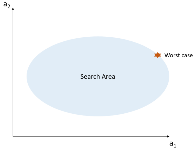
Figure 2.2: Robust Optimization: the area in this graph represents the set of value the parameters a_1 and a_2 are assumed to belong to. The star identifies the combination of those parameters that causes the worst impact on the system performance.
