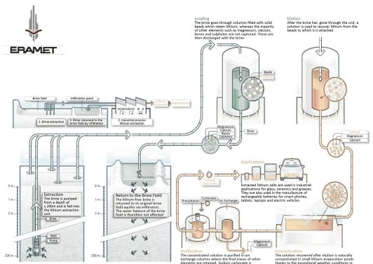
added to precipitate lithium in the form of lithium carbonate
