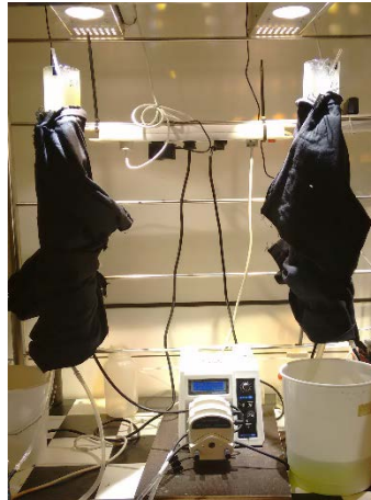
Figure 3-6 Picture of the two parallel photobioreactors covered with a black sheet and the lamps on the top
