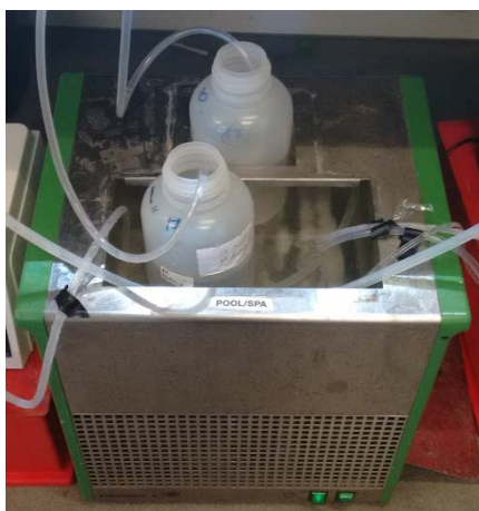
Figure 3-8 Cool system for influent storage
