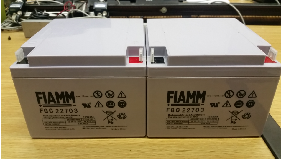
Figure 5.2: FIAMM FGC 22703 rechargeable lead acid batteries.
