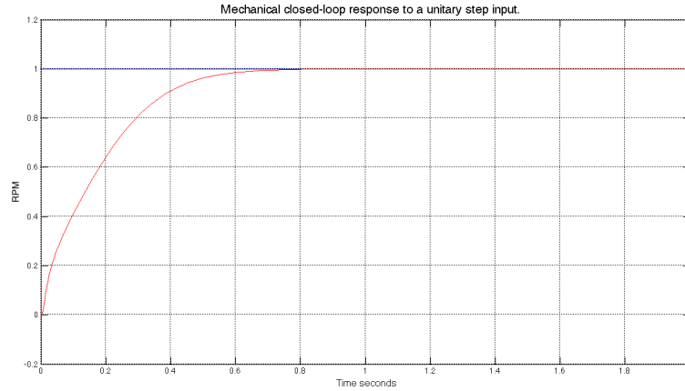
Figure 4.3: Mechanical closed-loop response to a unitary step input.
