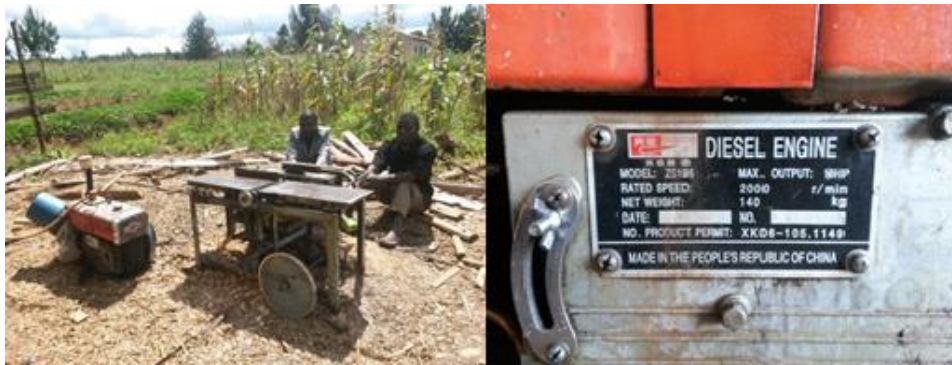
Figure 3-9 Cutting Wood machine fueled by Diesel engine (left); Diesel Engine technical features (right)
