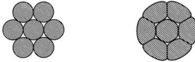
Figure 13: Standard and compacted 7-wire prestressing strands (Source: Nawy, 2009)
