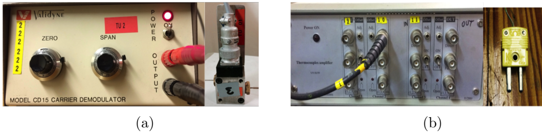
Figure 2.6: Validyne amplifier with differential pressure transducer (a) and Thermocouple amplifier with K-type thermocouple (b)
