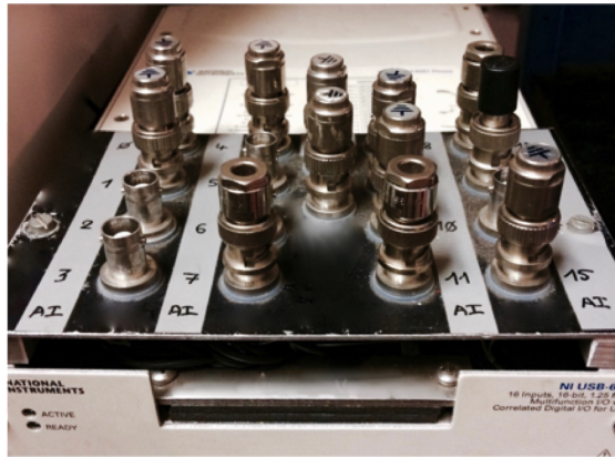
Figure 2.7: 16-bit National Instrument Acquisition System
