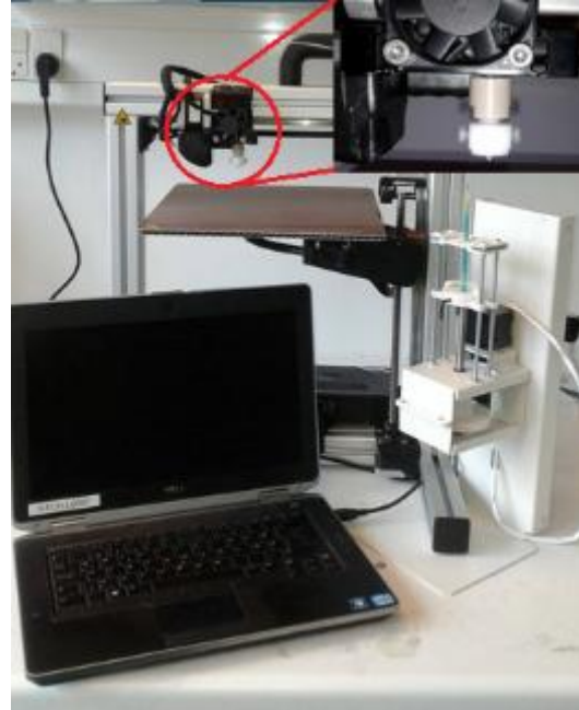
Figure 8 Mechanical set-up used during the project. From the left: the computer, the 3D printer and the paste extruder
