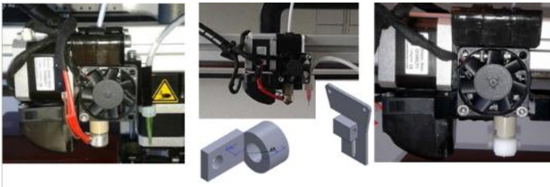
Figure 15 The three generations of the tip's holder. Starting from the left: the first, the second and the third one.
