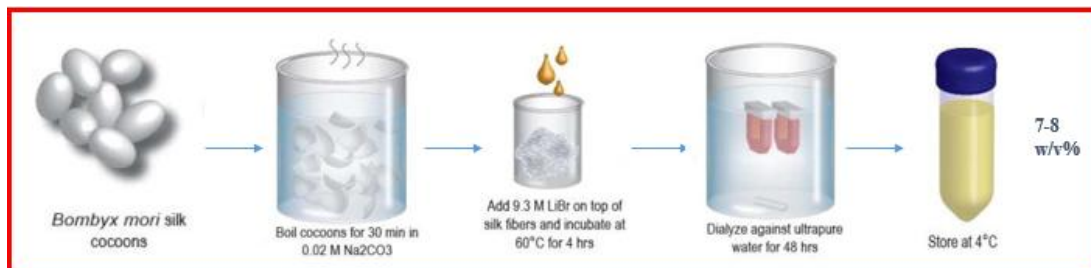
Figure 18 Schematic of the silk fibroin extraction procedure. Starting from the raw material (cocoons) to the final aqueous-based 7-8 w/v% solution will take 4 days [55]
