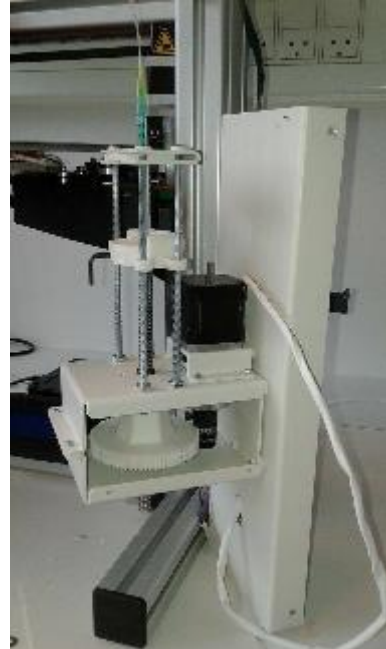
Figure 11 The Discov3ry universal paste extruder
