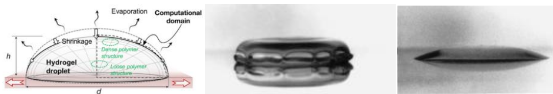
Figure 25 . Starting from the left: Schematics of a theoretical model of dropwise dehydration [64]; Impact of a molten wax droplet with velocity 0.8 m/s on an aluminum surface at temperature 23 °C (centre) and 73 °C (right) [61]
