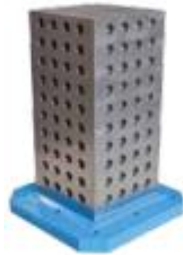
Figure 1.4 Tombstone with calibrated holes
