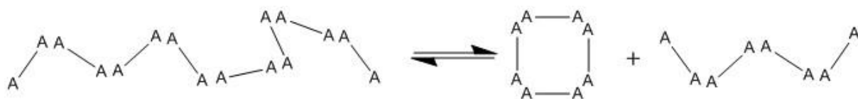
Figure 1.4.1 Example of ring chain equilibrium: a long linear chain is in equilibrium with its cyclic configuration together with the smaller linear part of it.
