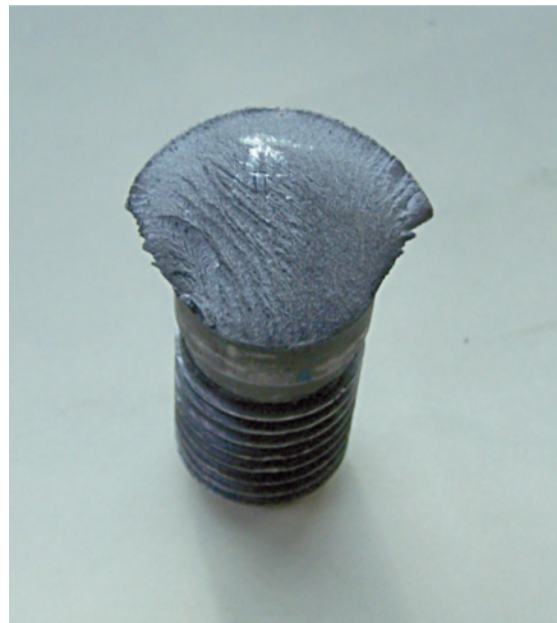
Figure 1.19: Hydrogen embrittlement and failure of a hard chromium-plated chain conveyor bolt.
