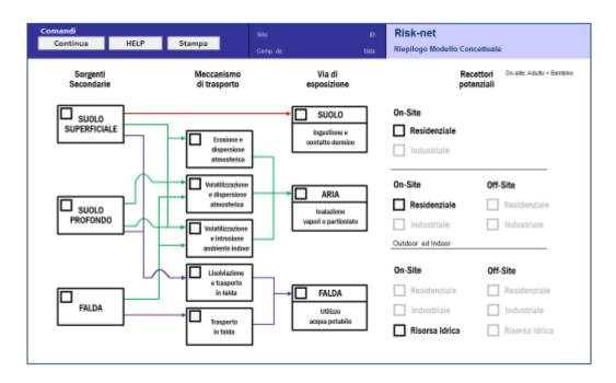
Figure 28: Schematic representation of the conceptual model of the simulation.
