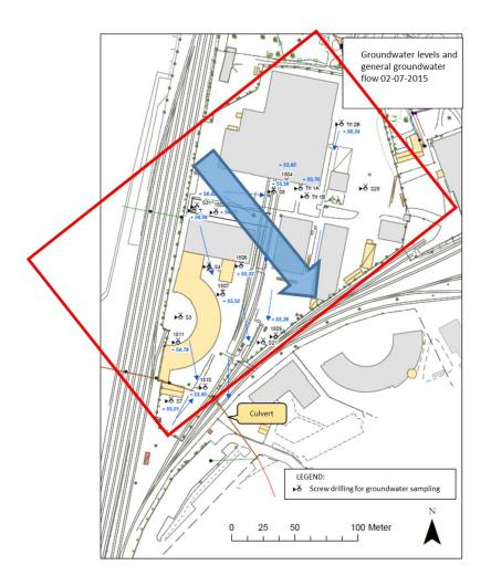
Figure 65: The blue arrow represents the plausible direction of groundwater flow and the red rectangle the schematic geometry representing the dimensions of the polluted site for groundwater matrix (Engström and Örne, 2015).
