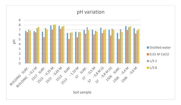
Figure 69: Soil pH variation before and during leaching test in the analyzed samples.
