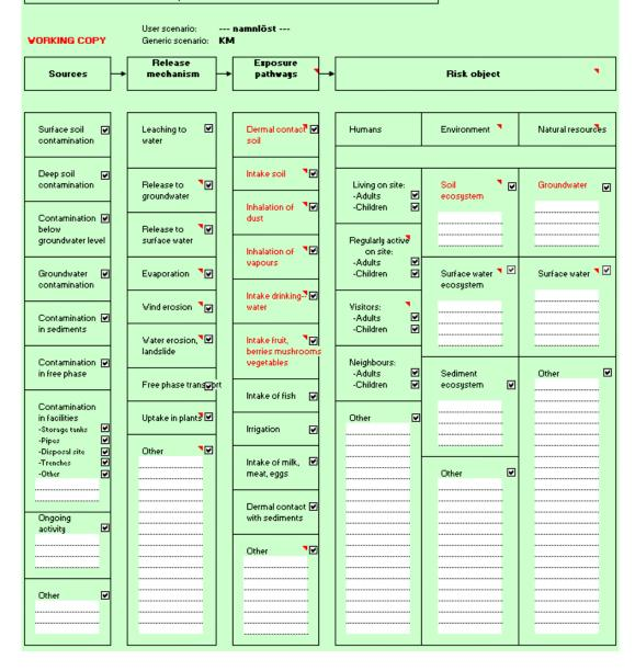
*Figure 42: "Conceptual model" sheet of the software for the determination of site-specific soil guidelines.*
