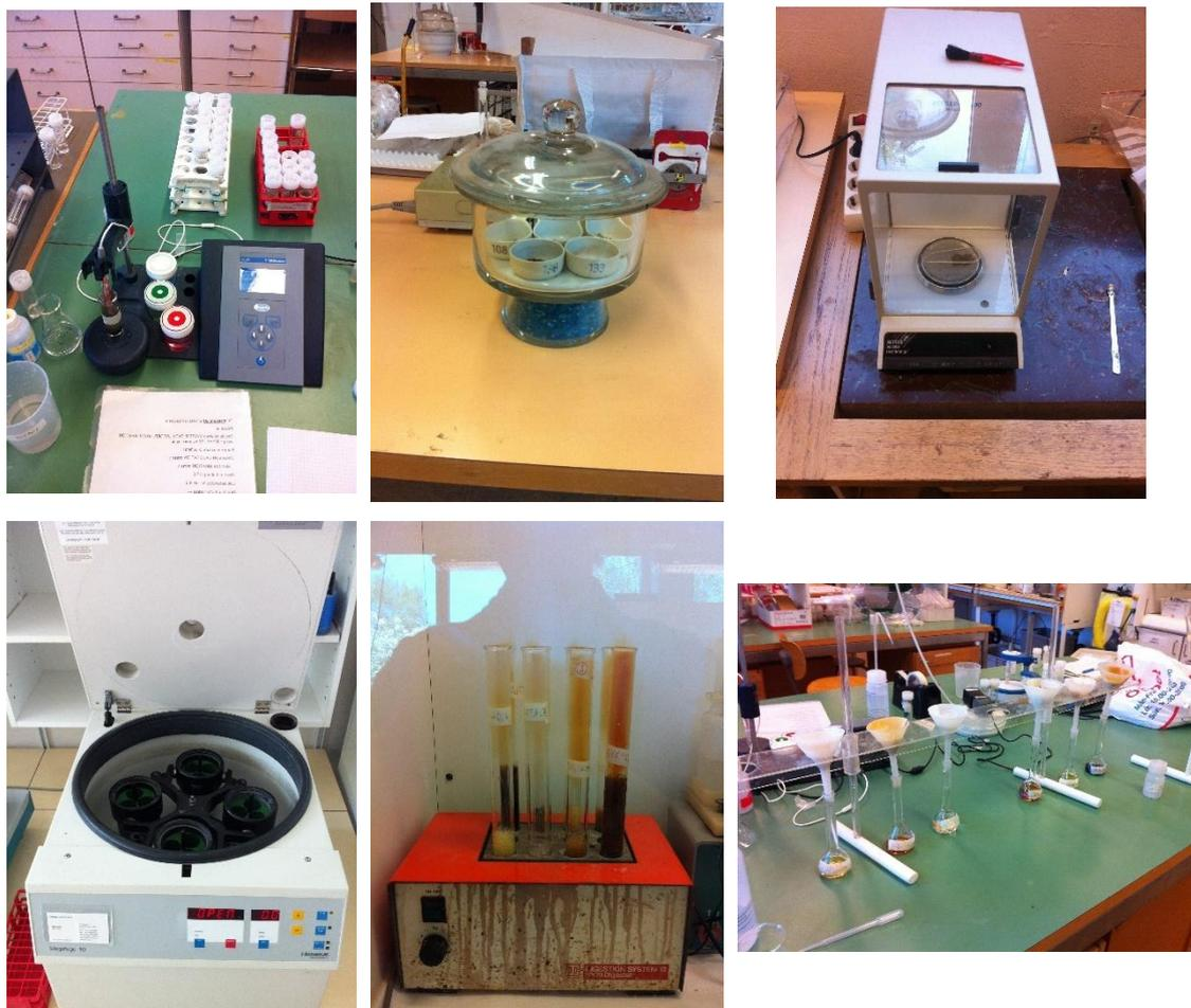
Figure 68: Part of the equipment used to perform the laboratory analysis. From the top-left, clockwise: calibrated combination electrode to determine solution pH; recipient for absorption of moisture of heated soil samples; high precision scale to weight soil samples; Acrodisc paper filters to filter the solution for total concentration of metals; plate for digestion of SOM; centrifuge for leaching test.
