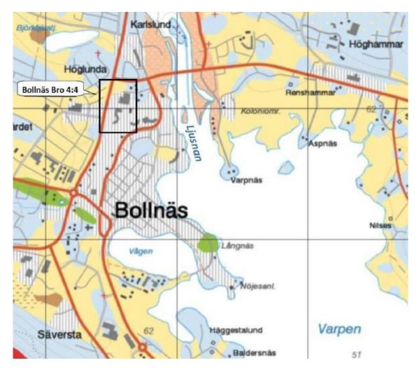
Figure 54: Geological map of the area of Bollnäs. The filling (striped area) covers the entire property of Bollnäs Bro 4:4 while the natural soil close to it is constituted by silt (yellow area) and moraine (blue area) (Engström and Örne, 2015).
