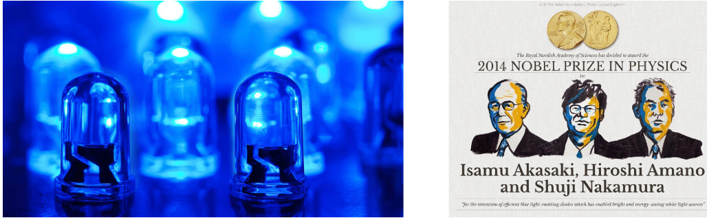
FIGURE 1.10: Blue LEDs using GaN as photoemitter allowed the production of white LEDs and the substitution of obsolete and more dissipative light sources.
