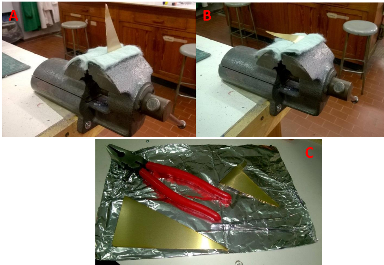
Figure 89 images of bending test procedures; fixing the sample(A), folding the sample(B), adjusting the bended piece (C).
