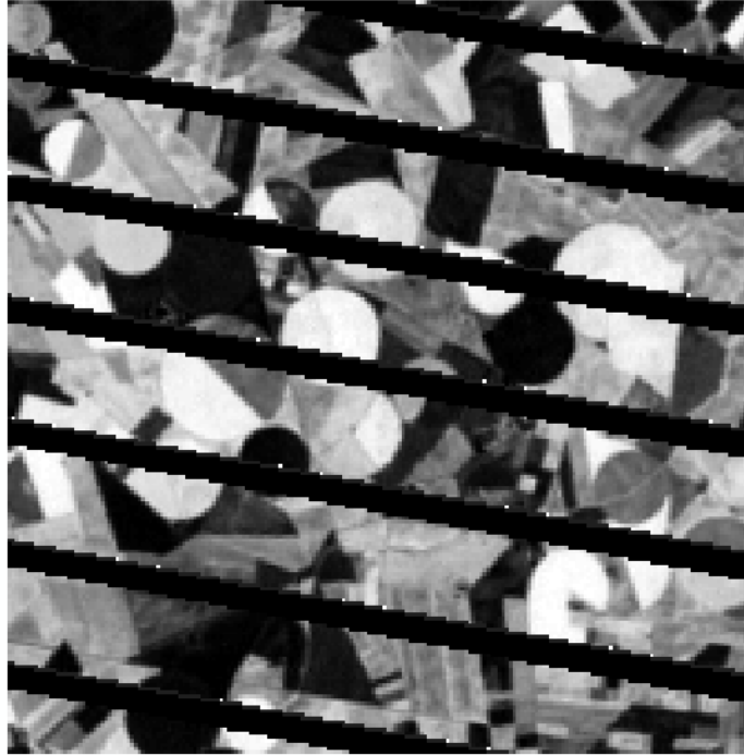
FIGURE 2. SLC LANDSAT 7 FAILURE IN THE IMAGERY OF THE 10 TH MAY 2011 IN BARRAX AREA
