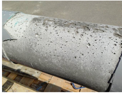
(c) Satisfying aspect of concrete once hardened and deshuttered.
