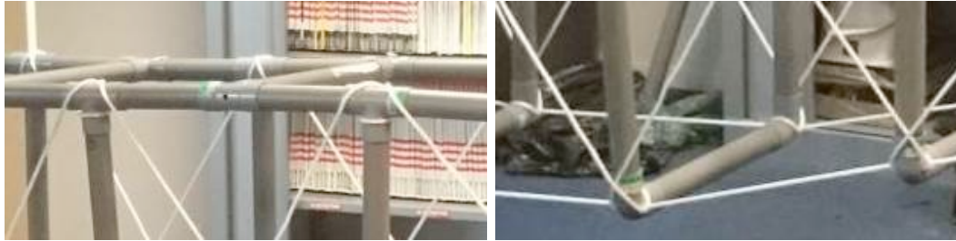
Figure 5.12: Sewing of the bracing rope along the longitudinal axis.
