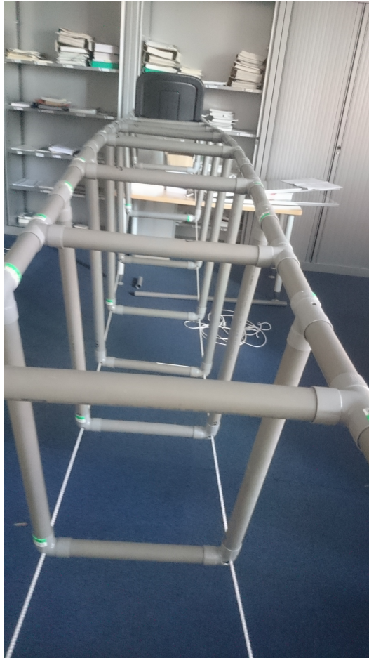
Figure 5.19: Stability: the footbridge is too deformable.
