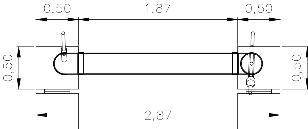
Figure 6.13: Section view of the concrete supports: from behind at the left, from the deck at the right.
