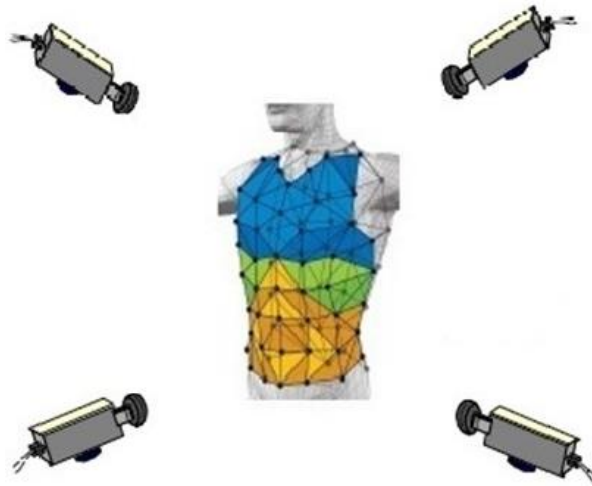
Figure 2.2.8.1.1 – Reconstruction of TV cameras and patient’s trunk. Black dots are markers placed on the patient and used as reference points.
