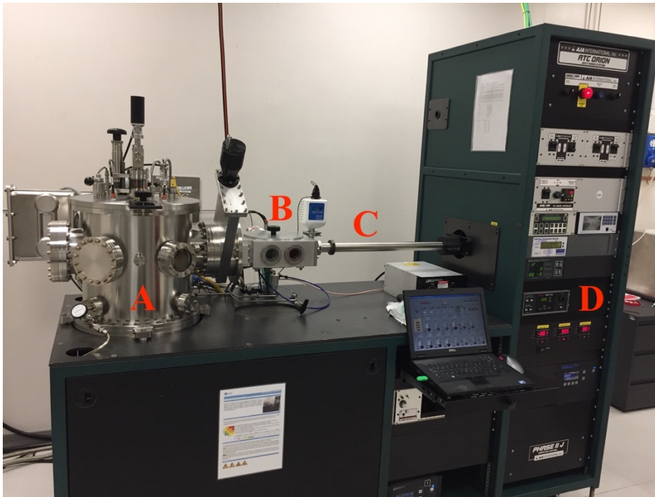
Figure 3.2: AJA ATC Orion magnetron sputtering system. (A) Deposition chamber. (B) Load-lock chamber. (C) Transfer arm. (D) Generators and controllers.
