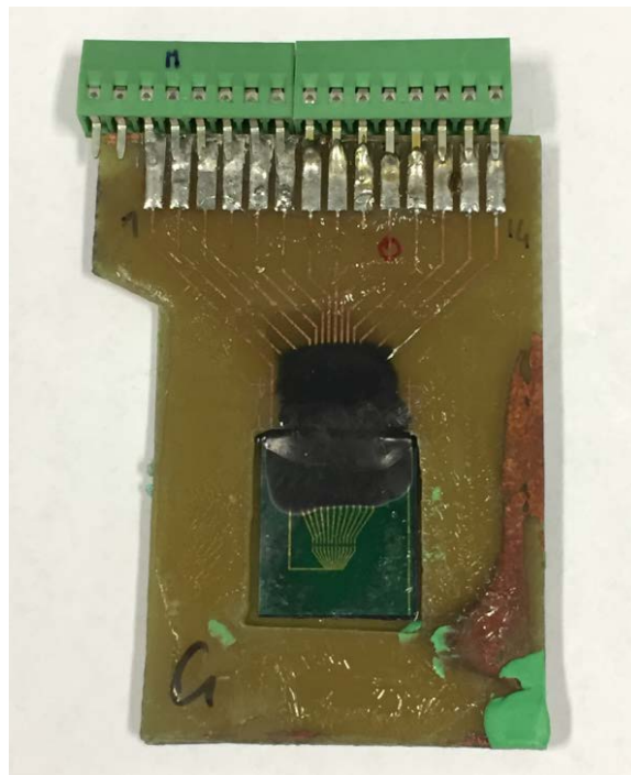
Figure 5.10: Chip bonded to the pads of the PCB. Then in order to protect the bonds from the biological environment, they were covered in a two-component epoxy. The hole, sealed with PDMS, is large enough to act as culture chamber itself.
