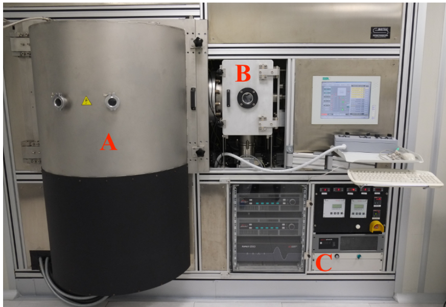
Figure 3.8: Ion Beam Etching Kenosystec VS80. (A) Main chambers. (B) Load-lock chamber. (C) Generators and controllers.
