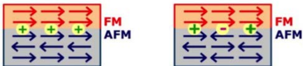
Figure 2.22: Spin configuration at a smooth ferromagnet-antiferromagnet interface in case of (left) uncompensated moment structure and (right) compensated moment structure.
