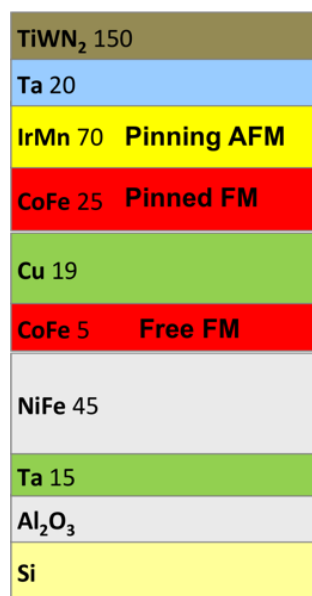
Figure 2.18: Sketch of the GMR-based sensor stack. Thickness in Å.
