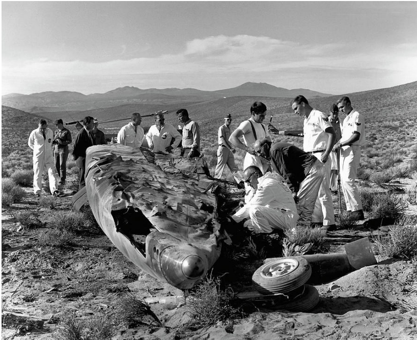
Figure 3.2: Crushed forward fuselage of North American Aviation X-15A-3 56-6672 (NASA).
