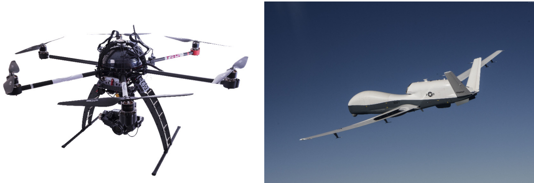
Figure 2.1: Examples of UAVs. On the left is shown the XM6 Qi-TR multirotor used for roof inspection. On the right is shown the Northrop Grumman MQ-4C Triton, built for the United States Navy as a surveillance aircraft.
