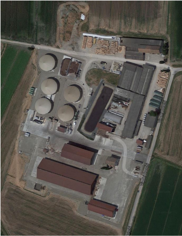
Figure 5-23: A view from satellite of “Azienda Agricola San prospero”. Four fermenters and one post digester are noticeable. (Source: Google Earth).
