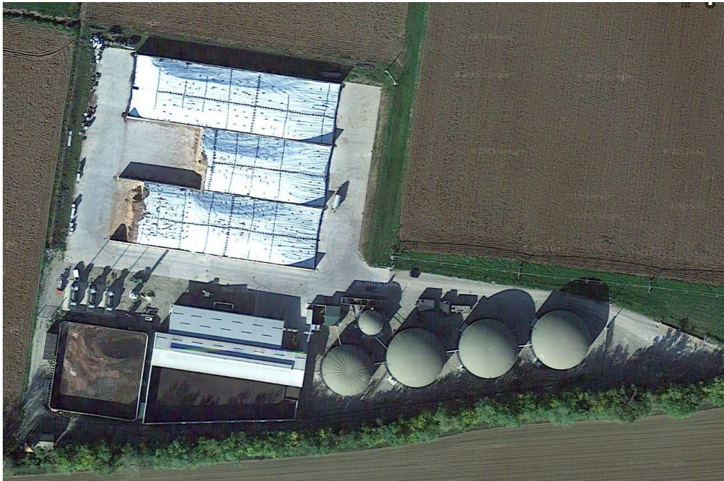
Figure 5-4: A view from satellite of “Valtrebbia Energia” Biogas Plant. We can see clearly the line digester, the storage area of crop and the three CHP units. (Source: Google Earth).
