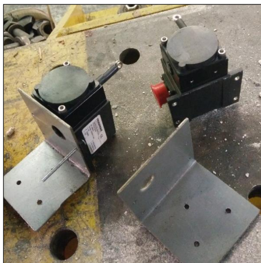
Figure 4-8. WDT instruments with their L shaped mounting elements
