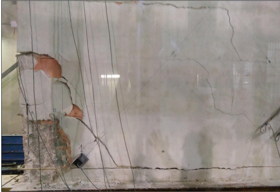
Figure 5-5. Cracks during the fourth loading cycle
