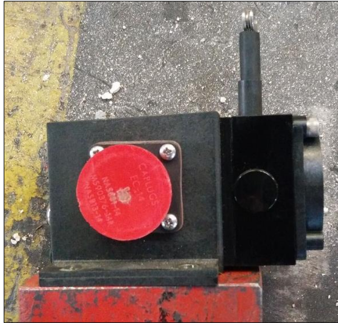
Figure 4-6. Wire Drawn Transducer used in the experiment
