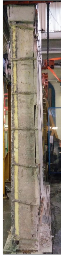
Figure 5-7. Out of plane damage during fifth cycle
