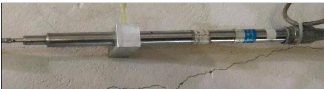
Figure 4-5. One of the LVDT transducers used in the experiment (already installed)
