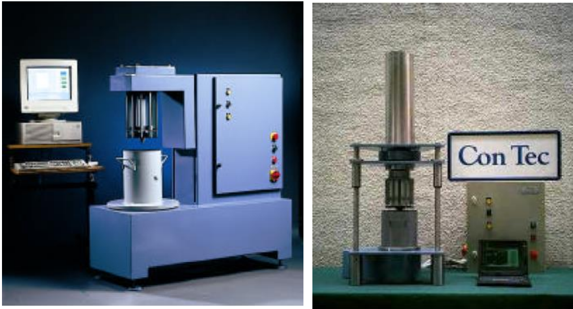
Figure 5. The ConTec viscometers, Version 3 and Version 4 3 . (Source: Banfill , 2000)
