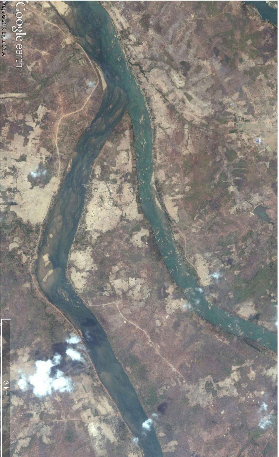
Figure A7: Se Kong-Sre Pok confluence during low flow conditions (20th March 2013). Different bed material of the two rivers is clearly visible. Bed rock steps and small bed-rock bars are abundant in the Se Kong River (Figure S8 and S9). Bed material in the Sre Pok is dominated by sedimentary bed-forms with a braiding pattern of the low for channel (Figure S10). These channel patterns continue downstream of the confluence.
