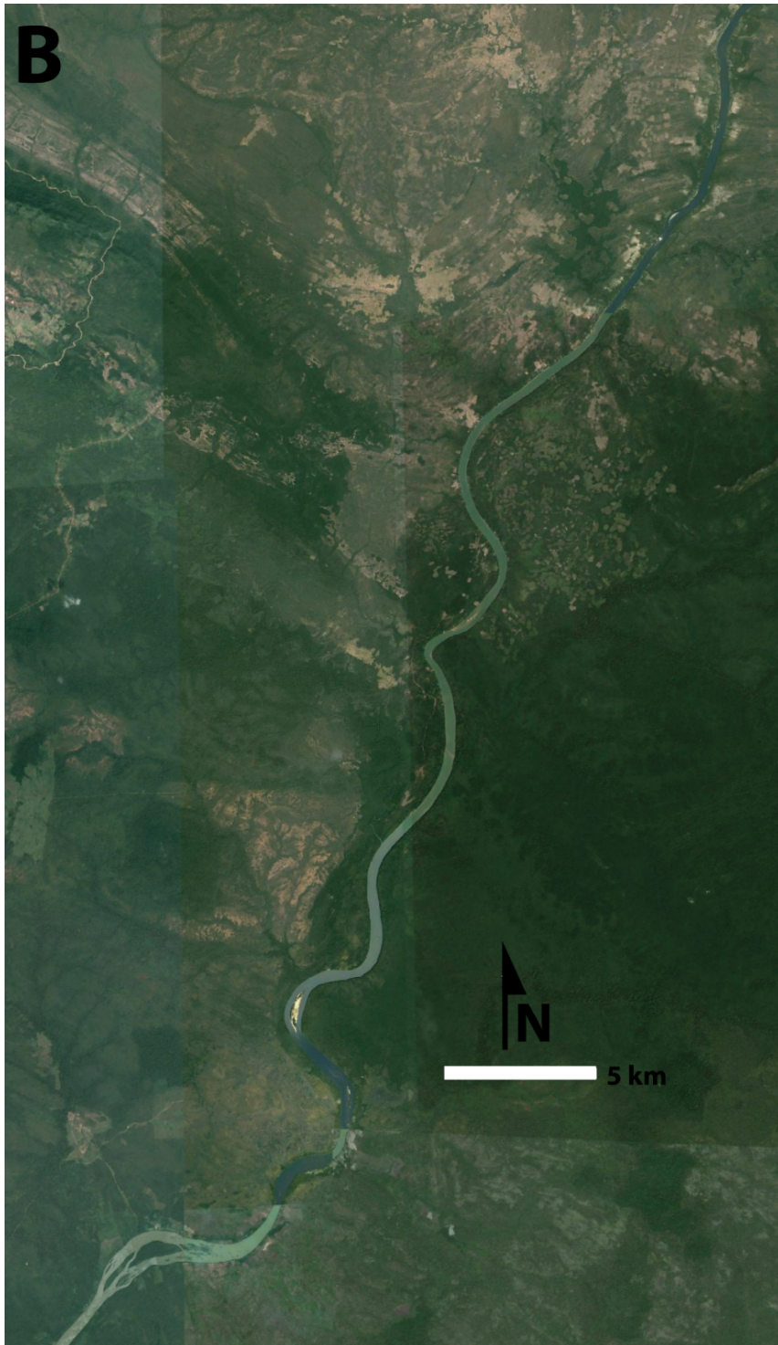
Figure A3: Middle Se Kong reach with decreased transport capacity. Transport capacities in this reach are lowest amongst all reaches in the 3S system. Visible fault systems in the upper part of the figure indicate the bed-rock control on this reach. Planform is straight, with no in-channel sediment deposits visible.
