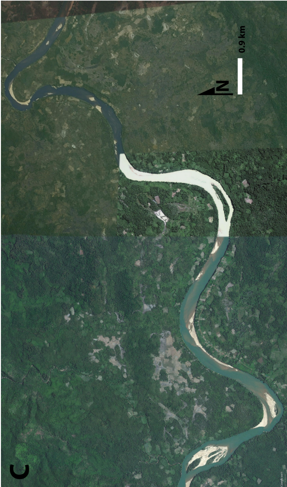
Figure A4: Middle Se San reach with decreased transport capacity. Platform is predominantly straight, but sediment deposits are visible in the channel and at several point bars.
