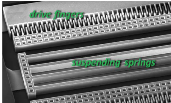
Figure 3.19: Detail of temperature-induced stress effects tolerant springs and comb-fingers for driving and sensing of the Tang resonator.
