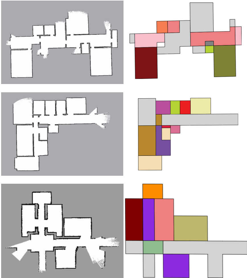
Figure 8.6: Examples of layout reconstruction from partial metric maps (partially explored rooms are in gray).
