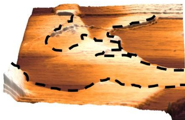
Figure 38. EC-STM ( 300 \times 300 \text{ nm}^2 ) image of HOPG graphite after a total pulse of 1.6 s at 1.2 V ( I_{\text{tunnel}} = 1 \text{ nA} ; V_{\text{bias}} = 0.3 \text{ V} ). The dashed black line emphasizes edge dissolution and HOPG swelling due to a blister (left-bottom corner).
