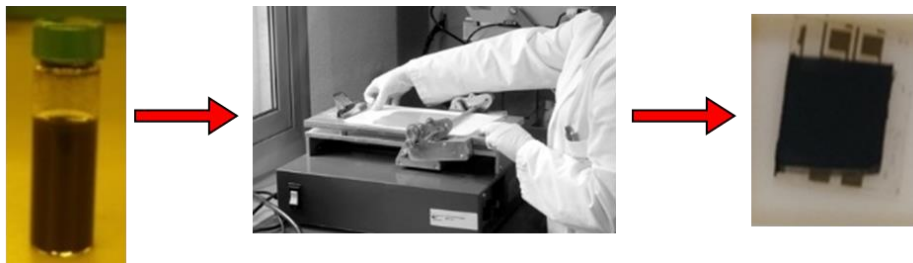
Figure 5-1 : a) Schematic of the synthesis of Printable Perovskite Particles (PPP) is shown. b) The PPP-ink is shown which is then bar-coated on pre-patterned electrodes to obtain uniform few micron thick PPP films.
