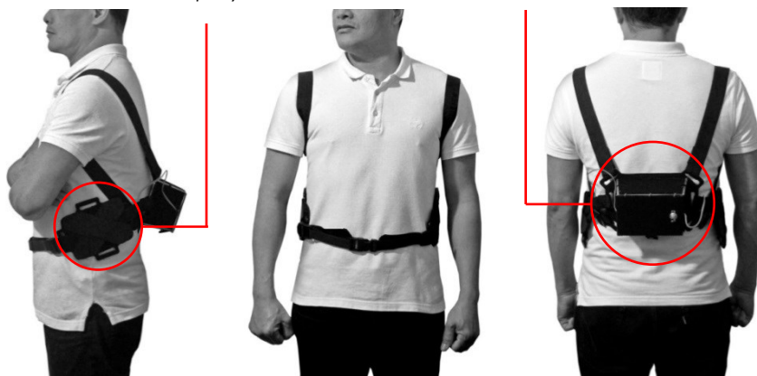
Figure 5.6: The positioning of the device's tactile display and hardware
