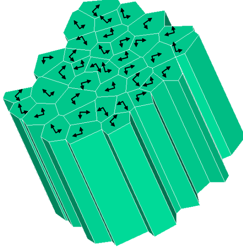
Figure 2.5: Digital realization of epitaxial polysilicon with identical out-of-plane axis and random in-plane orientation.
