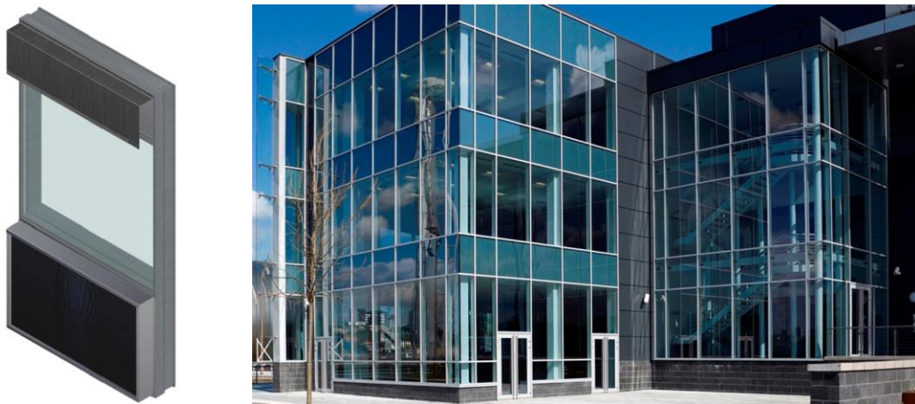
Figure 27 – 3D sketch of the unitized façade concept (left) (source: EURAC) and possible application result (right) (source: Metal Technology)
