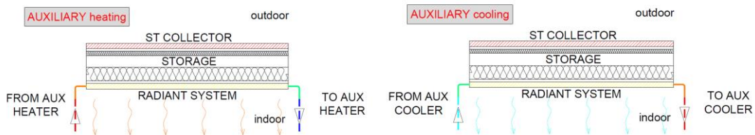
Figure 33 - Façade case study_Auxiliary Heating/Cooling layout
