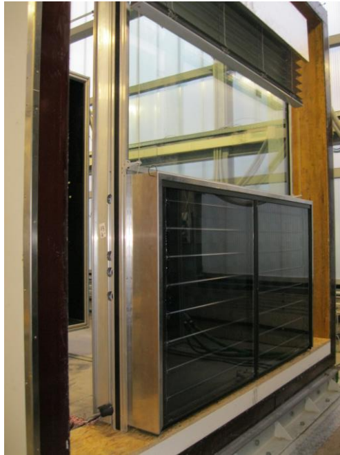
Figure 77 – Façade prototype installed within the INTENT frame: external side. The empty space around the specimen is filled with EPS blocks
