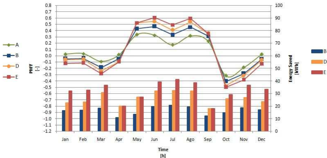
Figure 58. Comparison between Daily Average PMV variation and Thermal Energy reduction in Configuration 6 compared to Case A.
