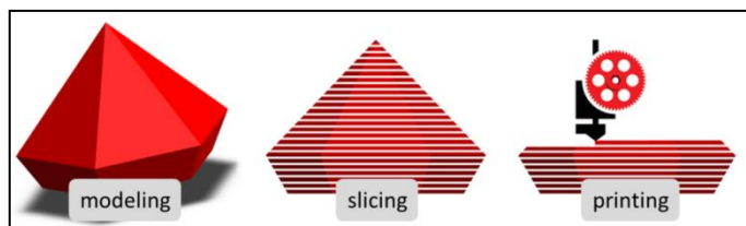
FIGURE 2.17 - SCHEMATIC REPRESENTATION OF THE MAIN PHASES NEEDED TO FABRICATE AN OBJECT.
