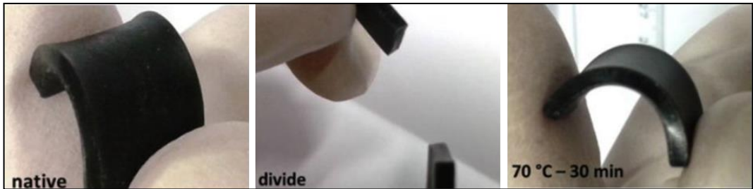
FIGURE 2.13 - ACRYLATE-BASED ELASTIC IONOMER SHOWING SELF-HEALING ABILITY AFTER A 30' THERMAL TREATMENT AT 70°C 34 .
