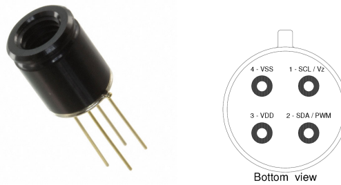
Figure 3.5: PIN description of MLX90621
