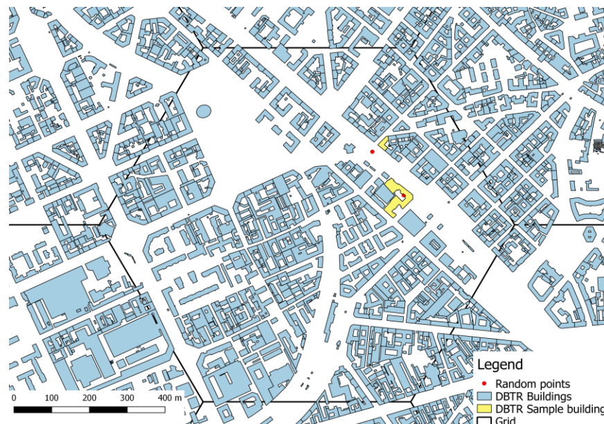
Figure 3.17 – Selection of the nearest building (yellow shapes) from the DBTR building layer respect to the random points (red points)
