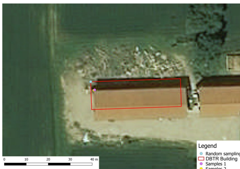
Figure 3.29 – Digitization of the corner (light blue dot) selected as reference in DBTR building (red shape) on the corresponding AGEA 2012 orthophoto corner (yellow and pink dots)
