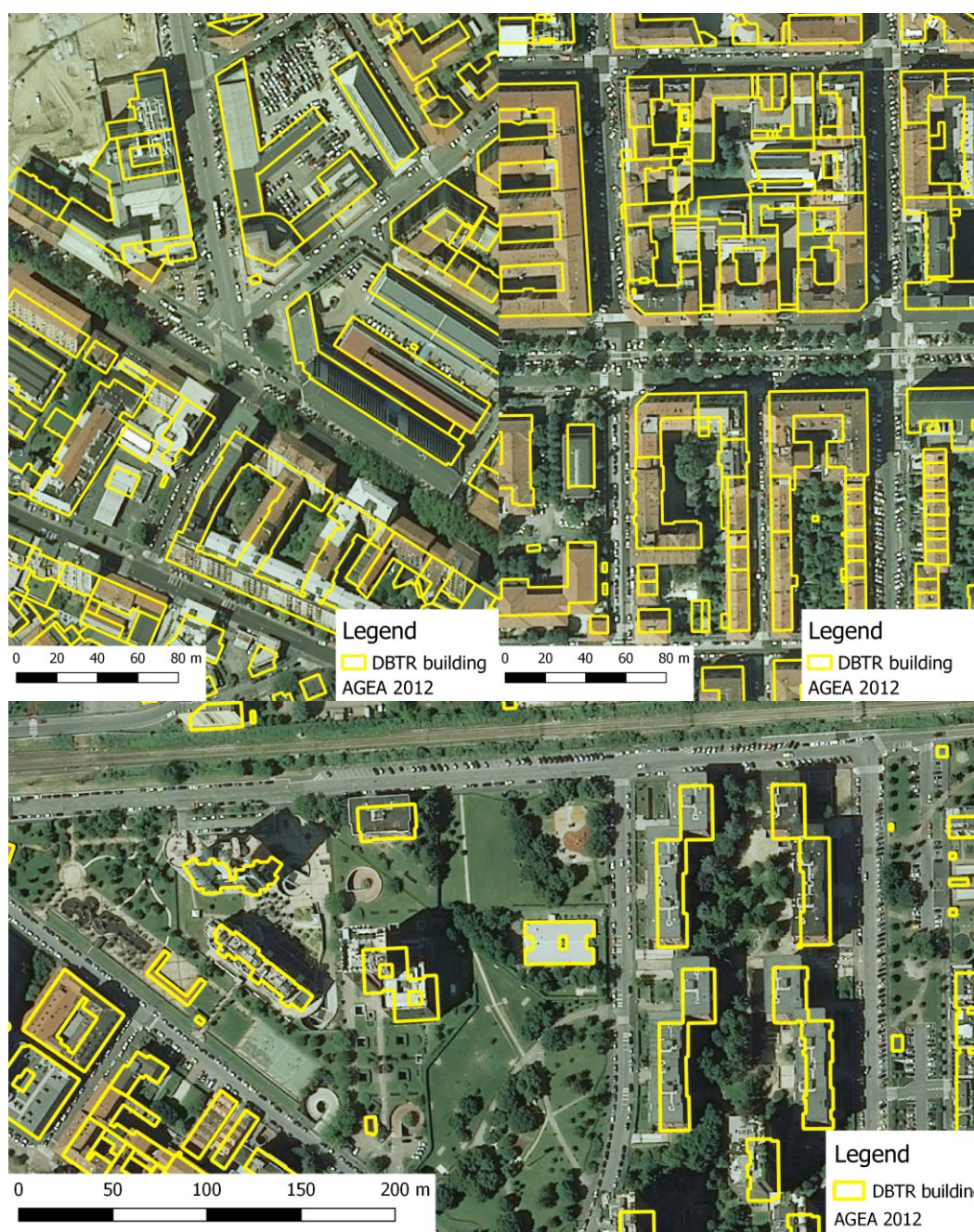
Figure 3.31 – Three example of visual comparisons between the AGEA 2012 orthophoto and DBTR building layer
