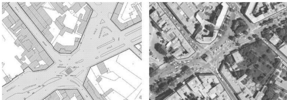
Figure 4.4 – Class Road area identification (left) respect to the equivalent area shown in an aerial image (right) (source: Topographic Database Technical Specifications)
