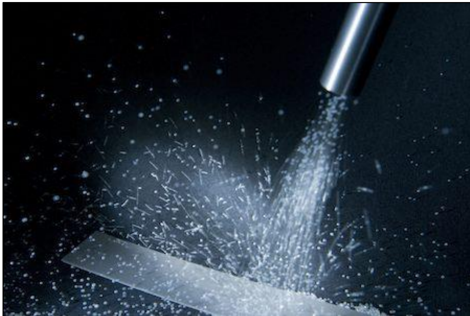
Figure 0.1 [2] – schematic of shot peening process
