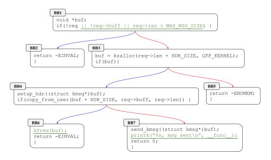
Figure 3.1: Control flow graph of the patched program from Figure 3.2.
