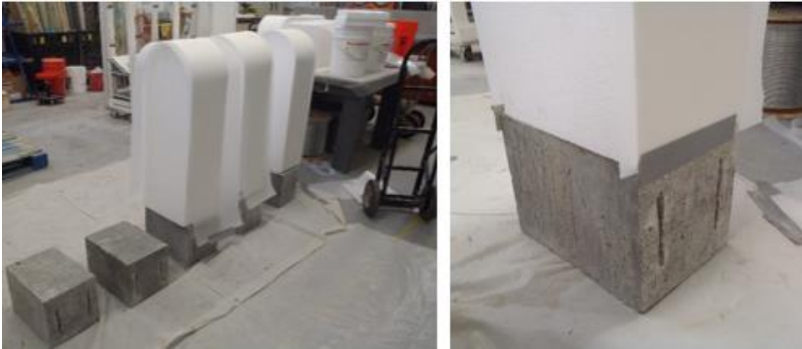
Figure 3.9 - EPS foam shapes assembling & Mylar installation
