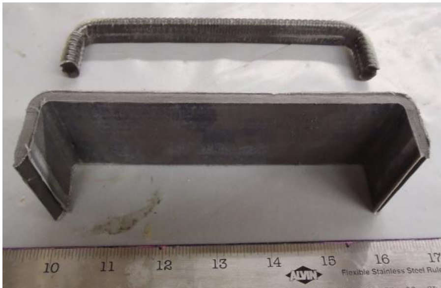
Figure 3.47 - Flat vs Round Staple anchor
