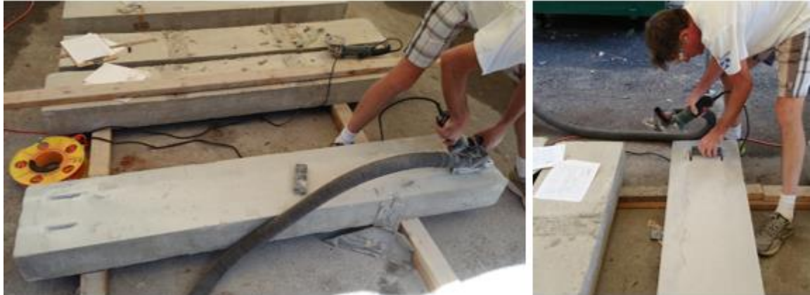
Figure 5.9 - Cutting Process specimens 001 & 002
