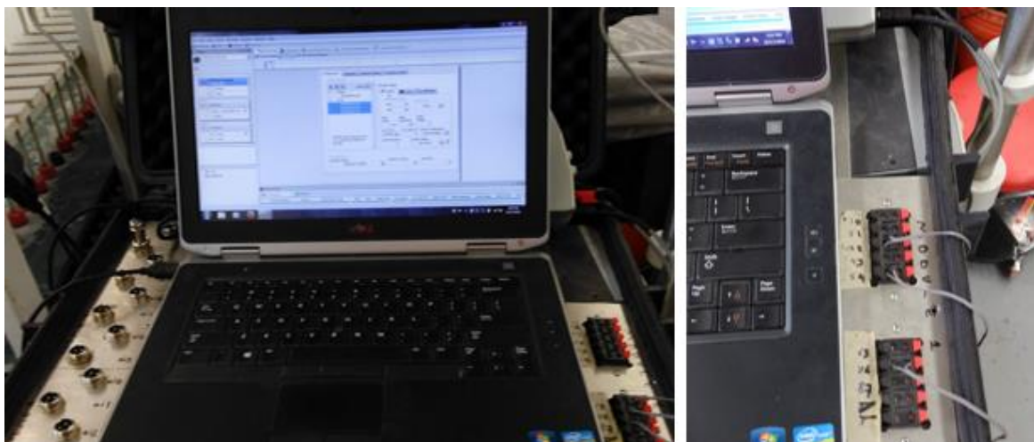
Figure 5.31 - Strain Gauges LVDTs and Load Cell connection
