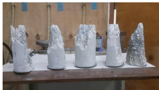
Figure 5.40 - Specimen after the compression test
