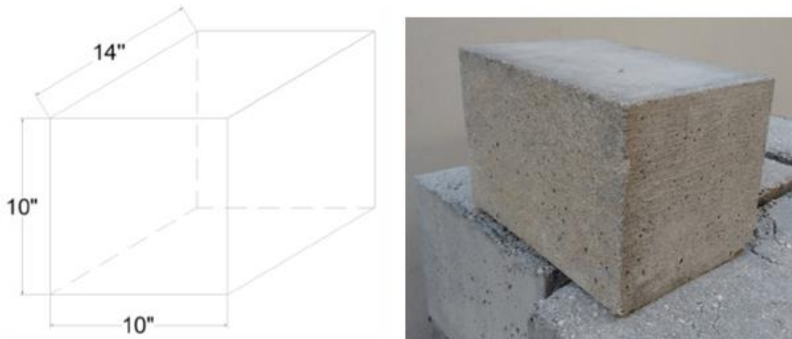
Figure A - Experimental Program 1 - Block's geometry
