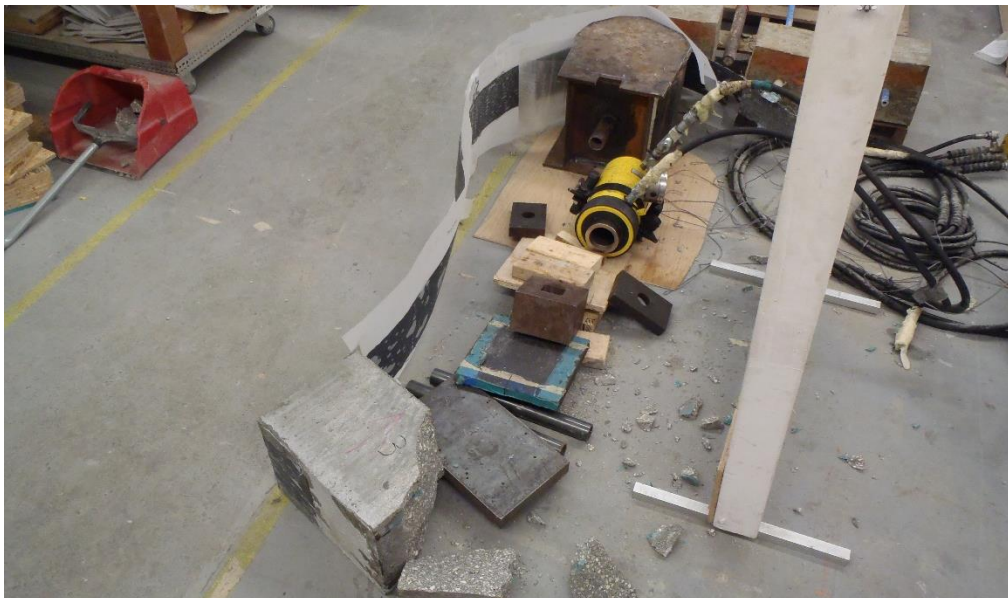
Figure 3.29 - Specimen failure at the end of the test
