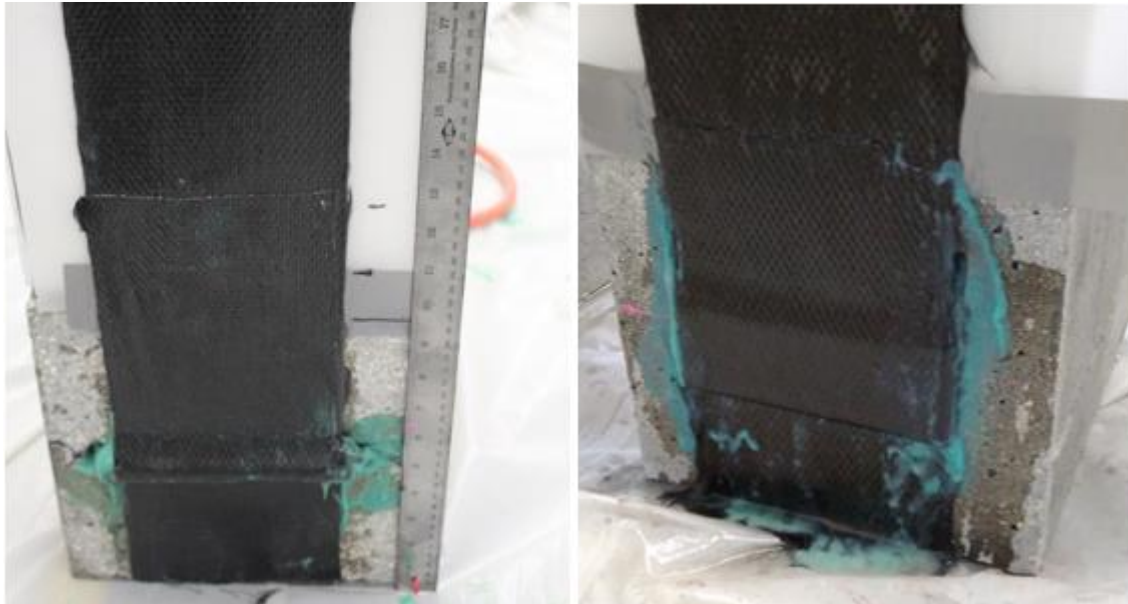
Figure 3.16 - Round Staple (left) & Flat Staple (right) anchor final product
