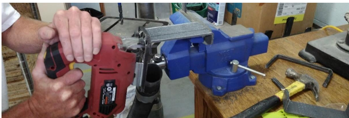
Figure 3.6 - Anchors' cutting process
