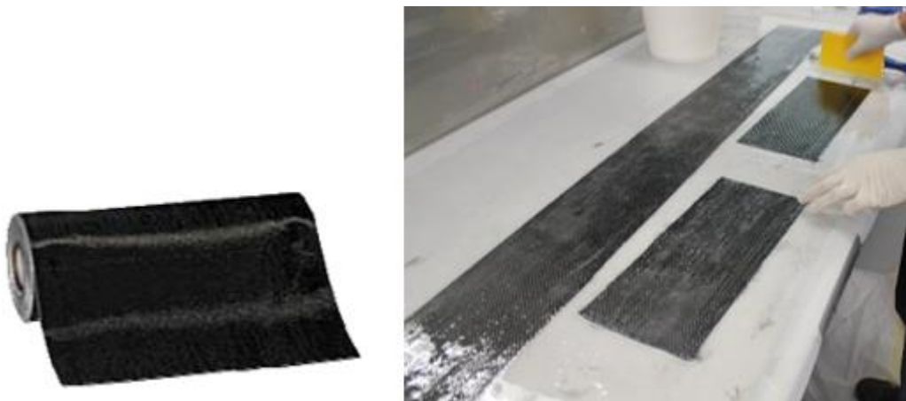
Figure 5.12 - V-Wrap C200H roll, 69" FRP sheet & 14" FRP patches
