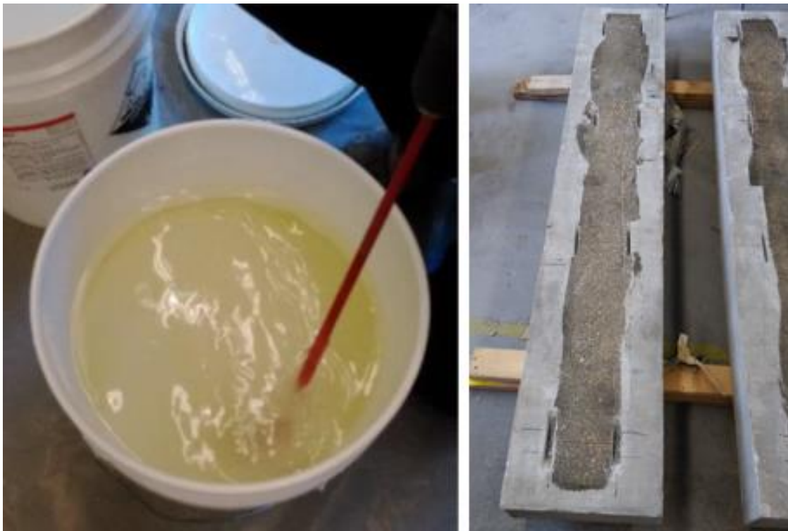
Figure 5.13 - Epoxy resin mixing & fume silica application on slab surface
