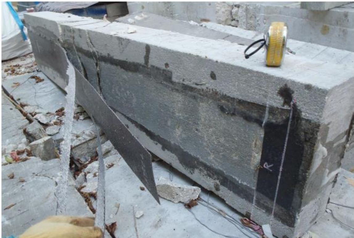
Figure 6.8 - C-FRP Specimen failure at the end of the test
