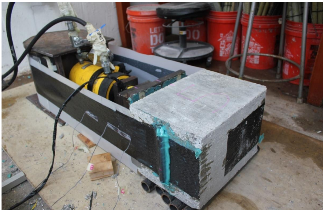
Figure 2.1 - Double Shear Test on a concrete block
