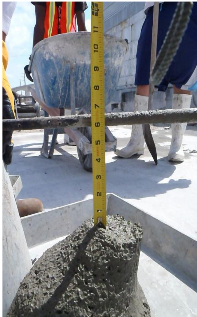
Figure 3.33 - Abrams Cone Slump Test
