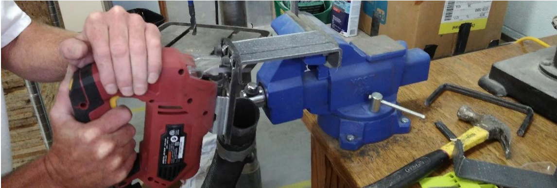
Figure 5.11 - Anchors' cutting process
