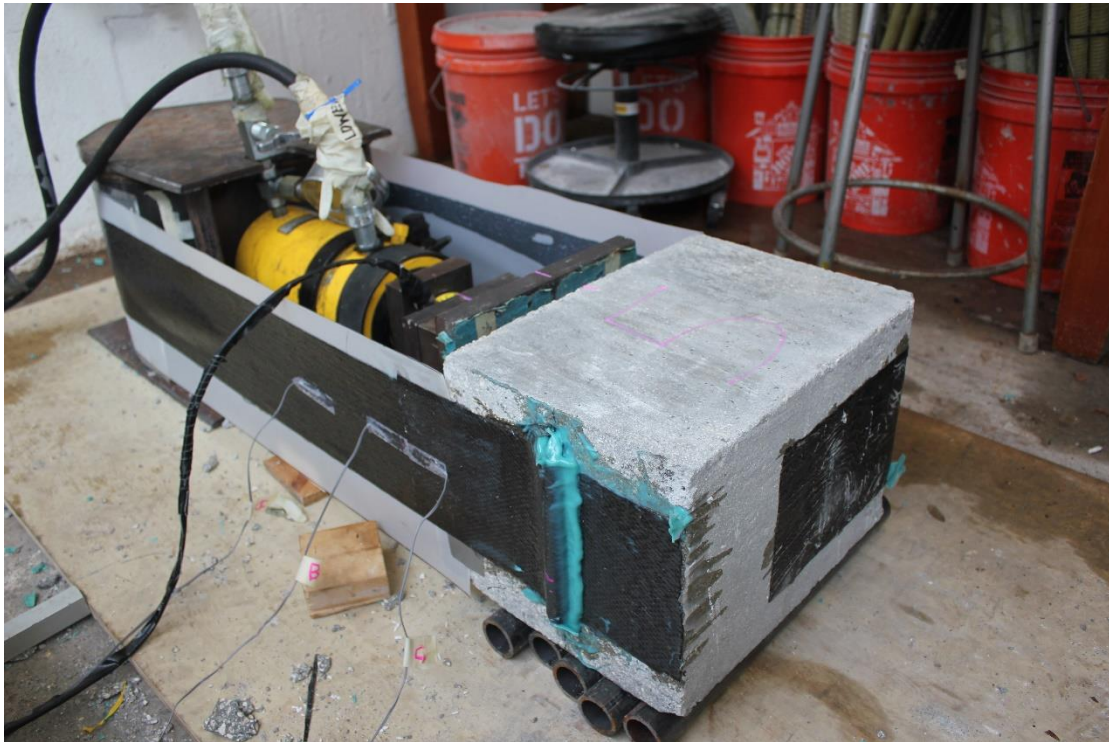
Figure 3.28 - Double Shear Test Set-up
