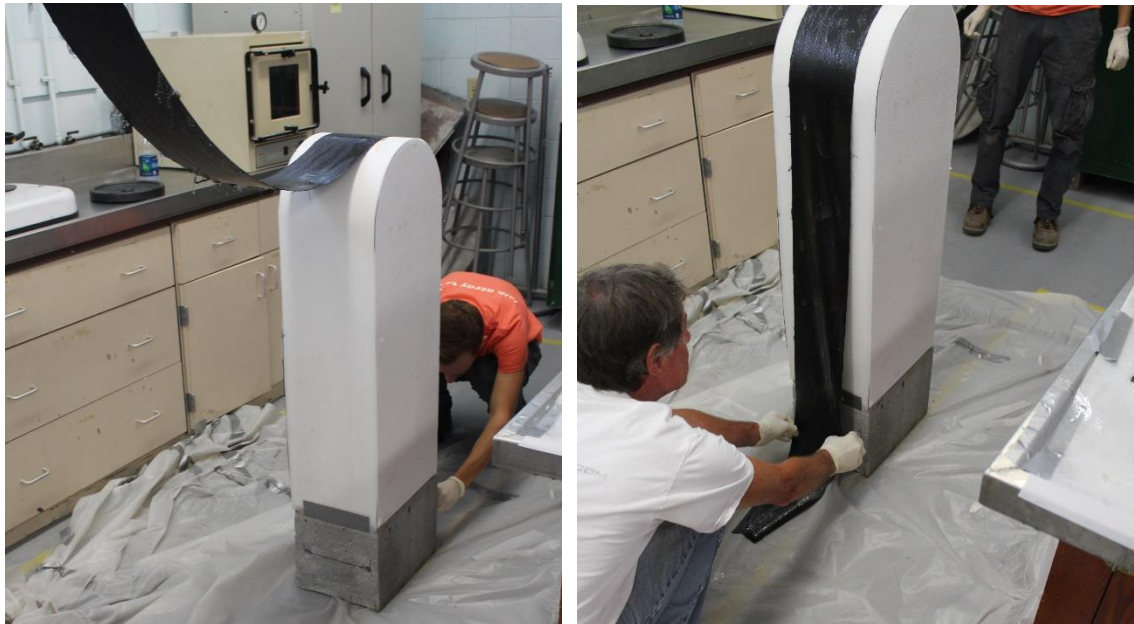
Figure 3.11 - Impregnated FRP sheet application
