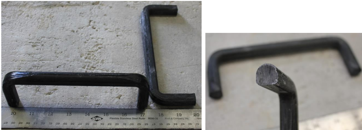
Figure 3.46 - Round Staple Anchor's Dimension
