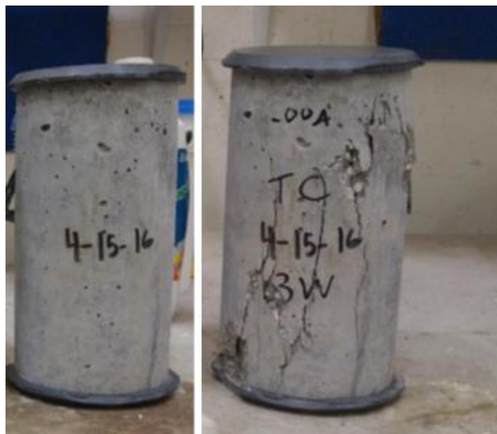
Figure 3.32 - Specimen before (left) and after (right) the compression test
