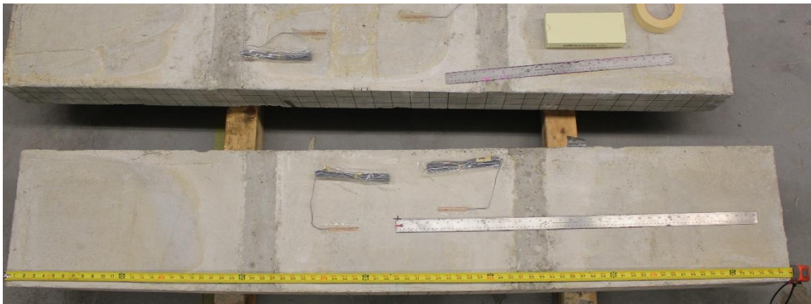
Figure 5.24 - Strain gauges on concrete
