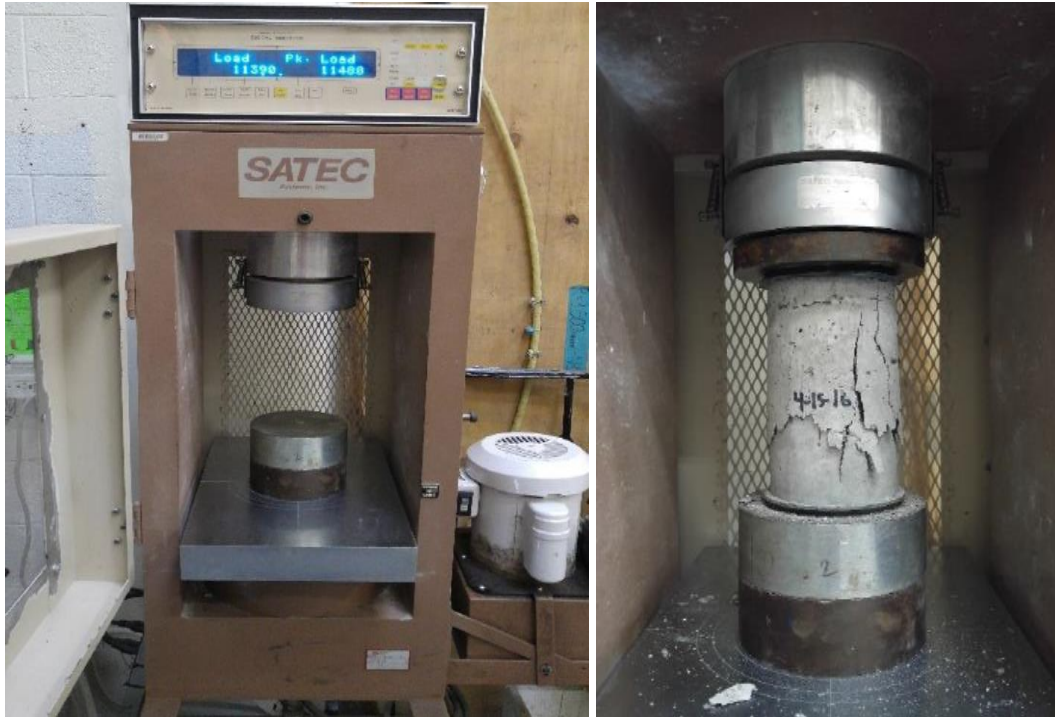
Figure 3.31 - SATEC (Compression Test Machine)
