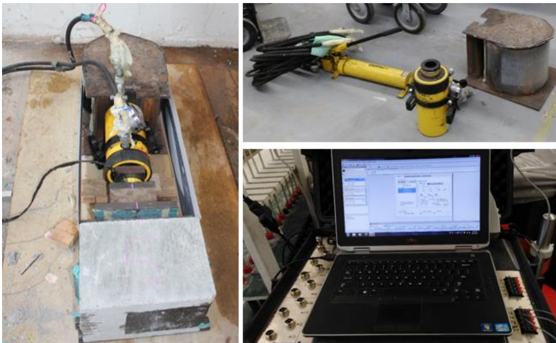
Figure 3.19 - Instrumentation used to perform the Double Shear Test
