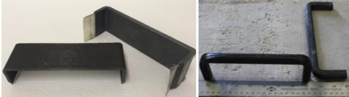
Figure 2.2 - Flat Staple (left) and Round Staple (right) anchors
