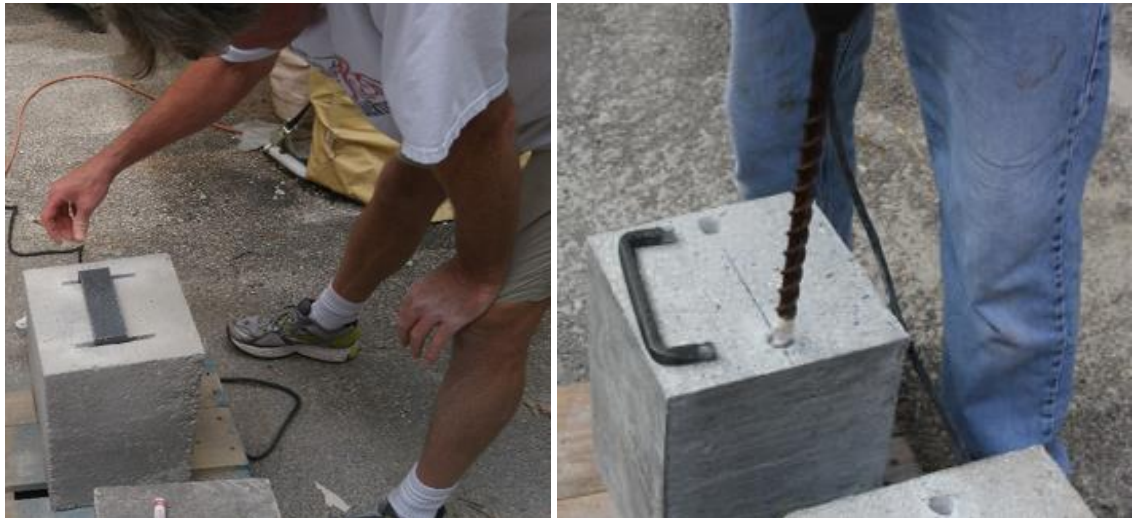
Figure 2.3 – Cutting and drilling process for anchors' installation
