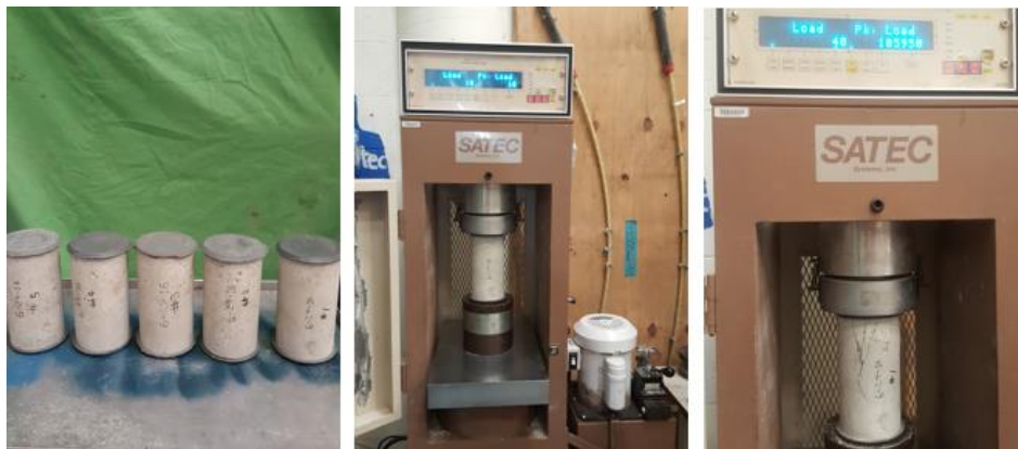
Figure 5.39 - Compressive tests on concrete cylinders
