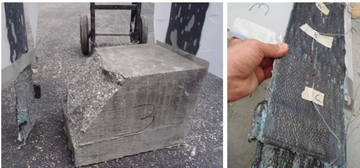
Figure 4.20 - Failure Mode F - Flat Staple anchor
