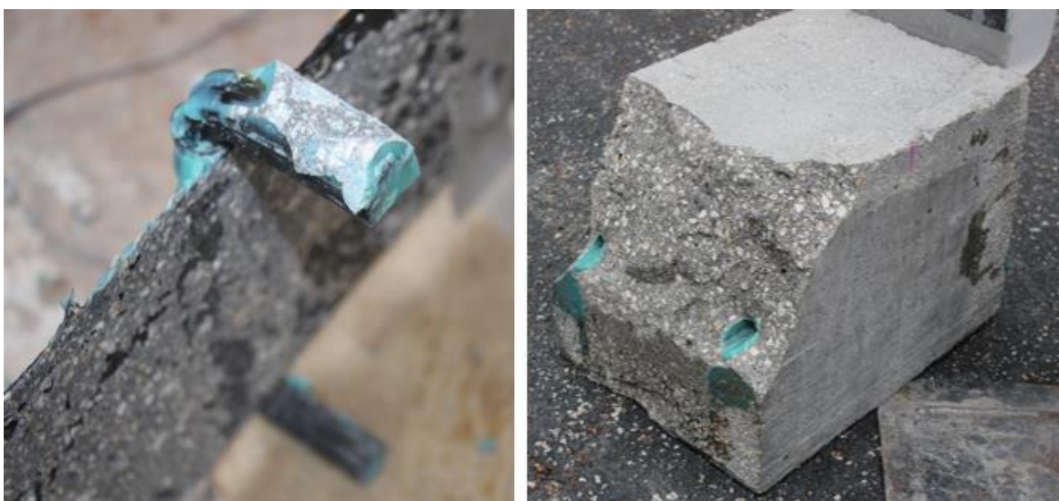
Figure 4.21 - Failure Mode F - Round Staple anchor
