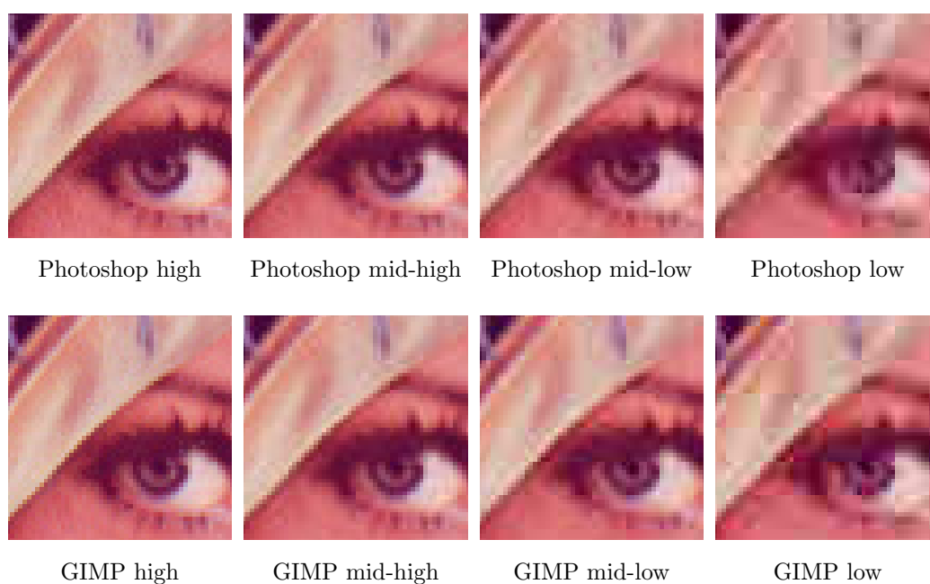
Figure 3.4: Different JPEG compression outcomes from different software products. Top: various Photoshop JPEG compression levels. Bottom: various GIMP JPEG compression levels.
