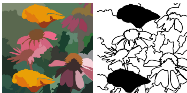
Figure 2.5: Example of regionwise tamper detection. Left: output of the segmentation algorithm; right: output of the tamper detector.
