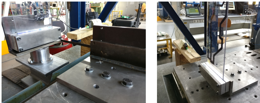
Figure 4.2: Real actuator connections - torsional modes excitation and flap-wise modes excitation
