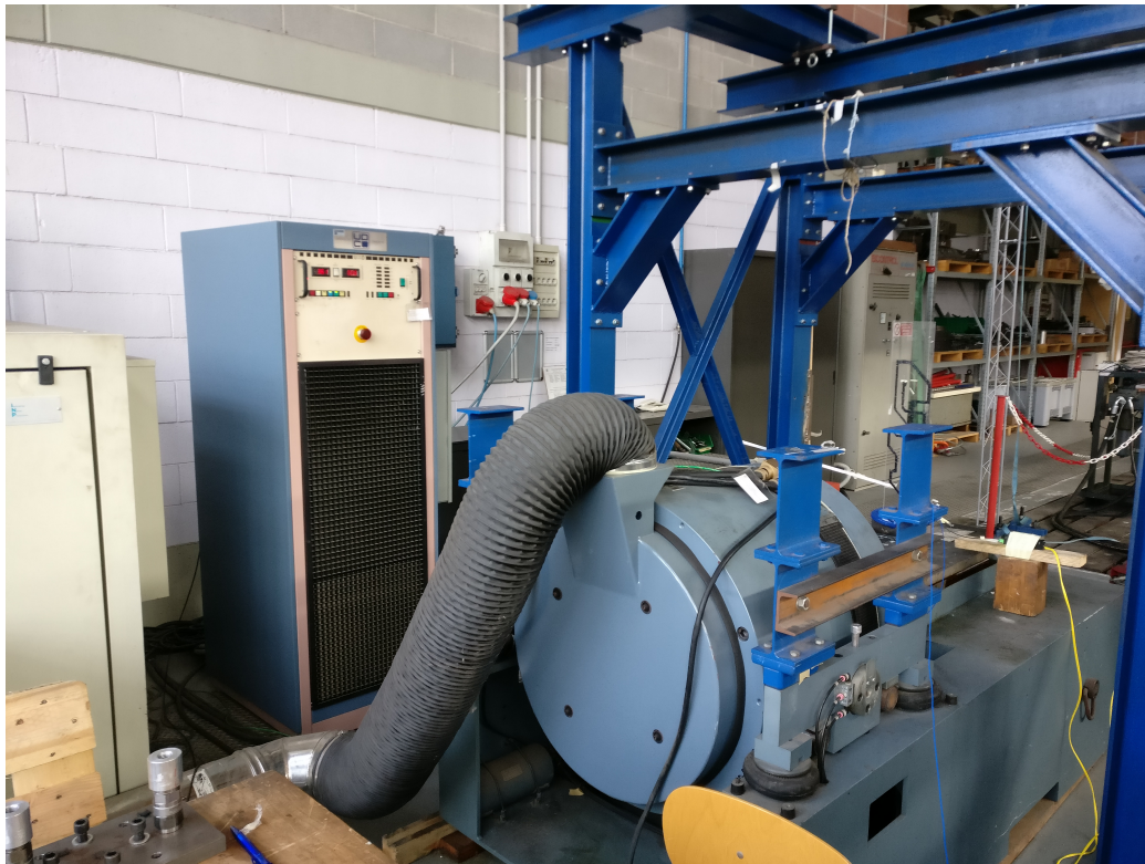
Figure 4.6: DM/PD005 Unholtz Dickie electrodynamic shaker
