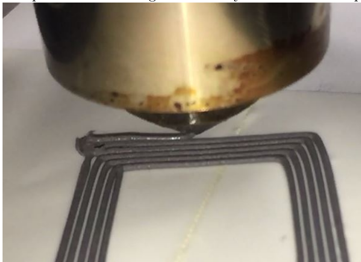
Figure 5.4: example of line breaking from one layer to the next: rapid movement
