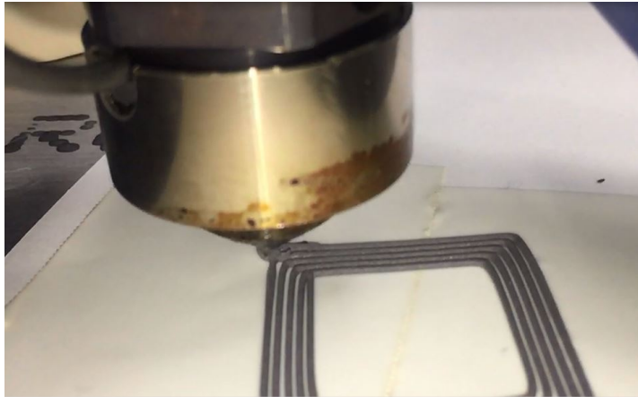
Figure 5.3: example of line breaking from one layer to the next: stop
