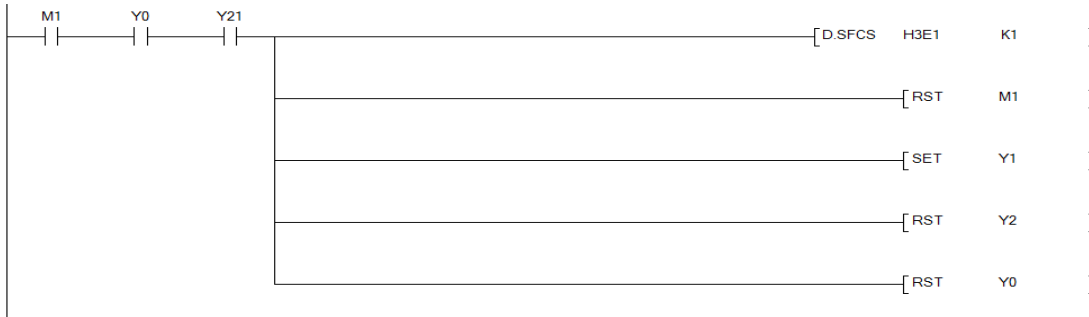
Figure 1.11: Ladder Diagram example
