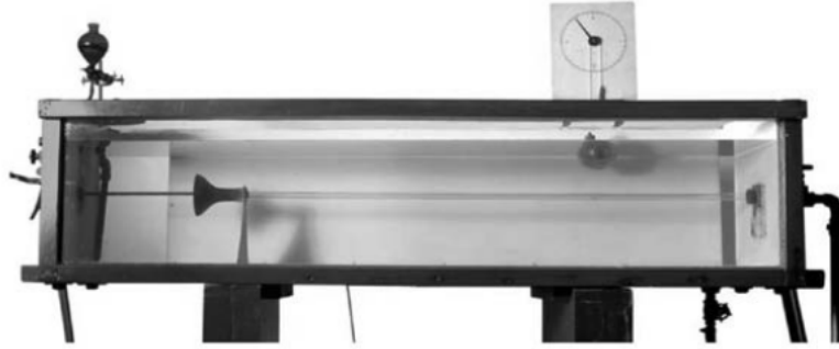
Figure 2.1: Osborne Reynolds' experiment asset used to observe the transition of the flow from the laminar to the turbulent regime [1].
